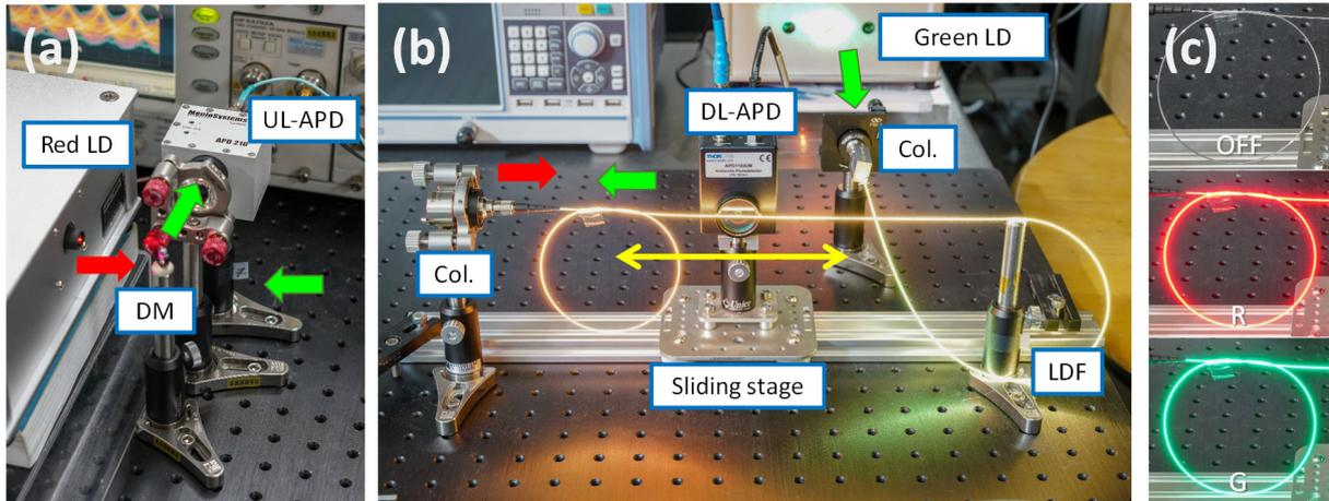
Fig. 3. Experimental photos of (a) head-end and (b) LDF optical antenna when both LDs are ON, and (c) LDF without and with red and green light launchings.
