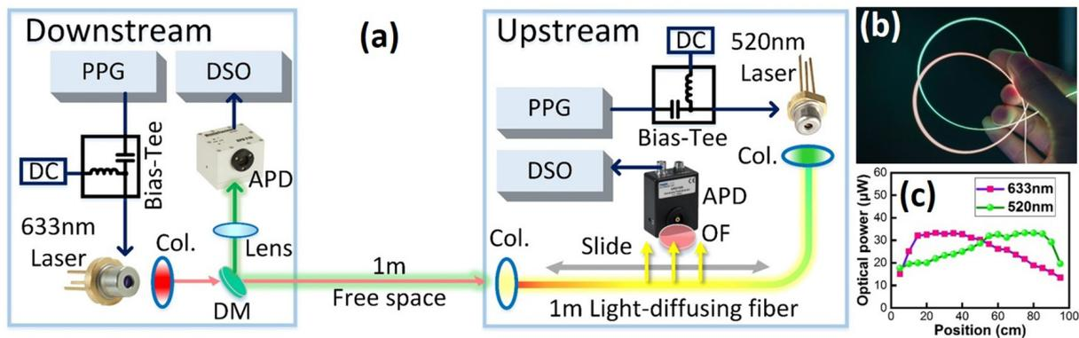
Fig. 2. (a) Experimental setup. (b) Photo of LDF and (c) measured power by a power meter at different fiber positions.
