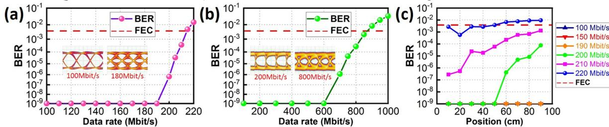
Fig. 4. Measured BER and eye diagrams in (a) the DL, (b) UL, and (c) DL at different data rates and at different position of the 100-cm LDF optical antenna.
