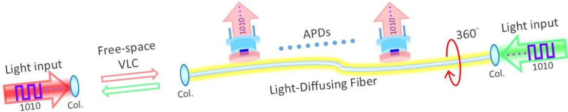
Fig. 1. Concept of using LDF as an optical antenna supporting multiple moveable Rx's.
