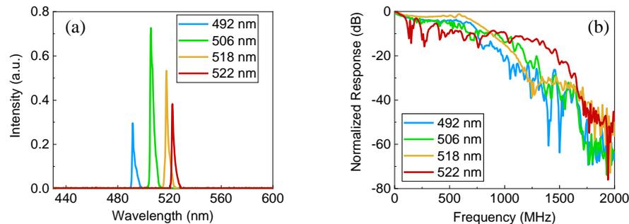
Fig. 2. (a) Optical spectra and (b) normalized frequency responses of four LDs with different wavelengths.
