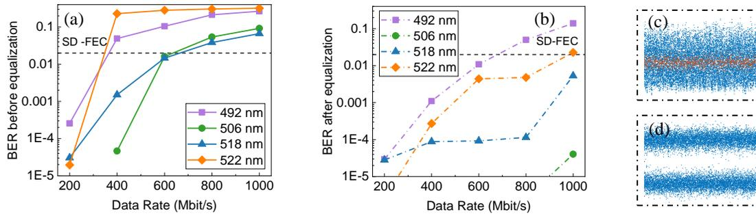
Fig. 3. BER versus different data rates for OOK modulation (a) before Volterra equalization and (b) after Volterra equalization. Signal amplitude distributions of 506 nm at 1-Gbit/s sample rate (c) before Volterra equalization and (d) after Volterra equalization.
