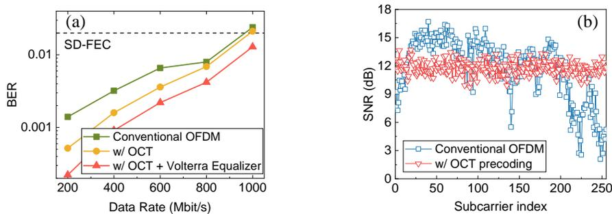
Fig. 4. (a) BER versus data rate for 8QAM-OFDM modulation, and (b) SNR profiles of the using conventional OFDM and OCT precoding at 1 GSa/s for 506 nm.
