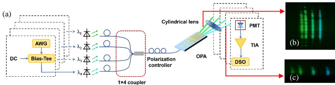
Fig. 1. (a) Experimental setup of OPA-based WDM system, (b) light spots before the cylindrical lens, and (c) light spots after the cylindrical lens.
