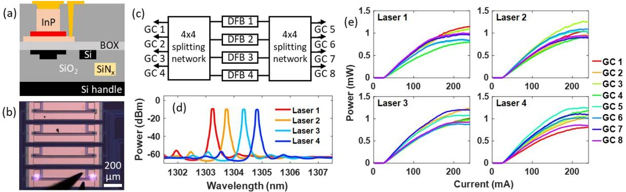
**Fig. 1.** (a) Cross section of the BSoBOX platform. (b) Die photo of the DFB laser array. The splitting network is located elsewhere on the chip. (c) Diagram of the DFB laser array. (d) Spectra from a laser array on die 3, at a common output GC. Each laser was measured individually, at 100 mA bias. (e) LI curves of the fiber-coupled power for the 4 lasers taken from all 8 GCs.
