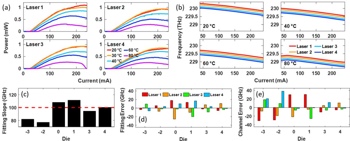
**Fig. 2.** (a) Fiber-coupled power vs. current for one output of the array. (b) Peak frequency vs. current for the  $4\lambda$  DFB laser array at elevated temperatures. (c) Best-fit laser array channel spacing, from linear regression over the peak frequencies of an array, at 100 mA bias. (d) Deviation between the individual peak frequencies and their best-fit channel spacing. (e) Deviation between the individual peak frequencies and a 100 GHz grid.
