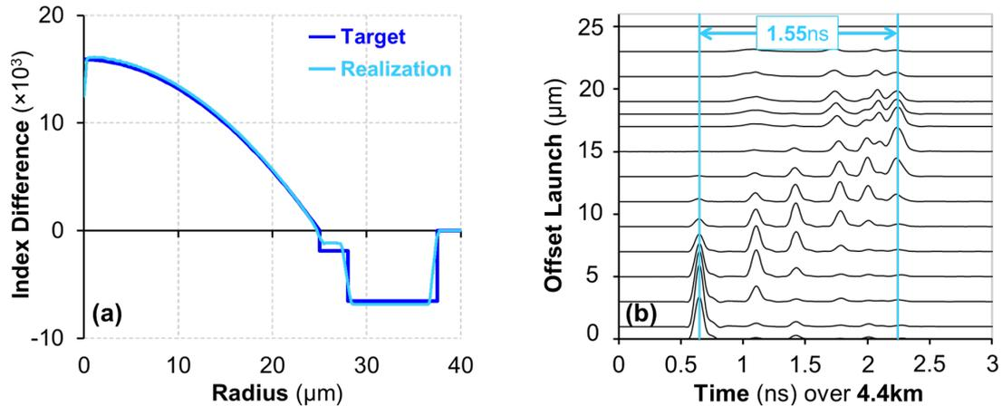
Fig.2: Experimental realization and theoretical target of index profiles of the 55-spatial-mode fiber (a); measured DMGD plot at 1550nm (b).
