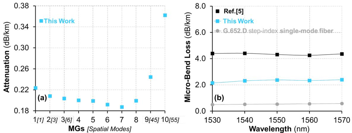
Fig.4: Measured attenuations at 1550nm as a function of the MGs for the 55-spatial-mode fiber [This Work] (a); measured micro-bend losses as function of wavelength for the 55-spatial-mode fiber [This Work], Ref.[5] and a standard G.652.D step-index single-mode fiber (reference) (b).
