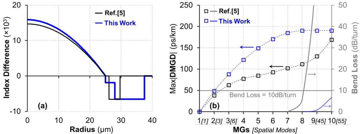
Fig.1: Theoretical targets of index profiles of the 55-spatial-mode fiber [This Work] and of Ref. [5] (a); calculated Max|DMGD| (open squares) and macro-bend losses at 10mm bend radius (solid lines) at 1550nm as a function of the MGs (b). Dashed lines are guides for the eye.
