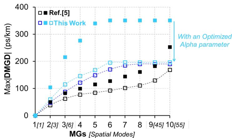
Fig.3: Measured (solid squares) and calculated (open squares)  $\text{Max}|\text{DMGD}|$  at 1550nm as a function of the MGs for the 55-spatial-mode fiber [This Work] and for Ref. [5]. Dashed lines are guides for the eye.
