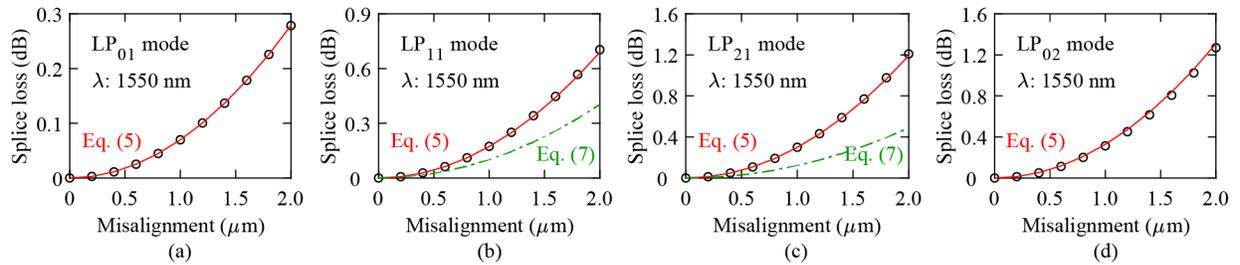
Fig. 2. Splice losses with respect to the axial misalignment for (a) LP $_{01}$ , (b) LP $_{11}$ , (c) LP $_{21}$ , and (d) LP $_{02}$  modes. Black circles represent the theoretical splice losses calculated by the overlap integral between the electric field. Red and green lines indicate the results estimated using Eqs. (5) and (7), respectively.
