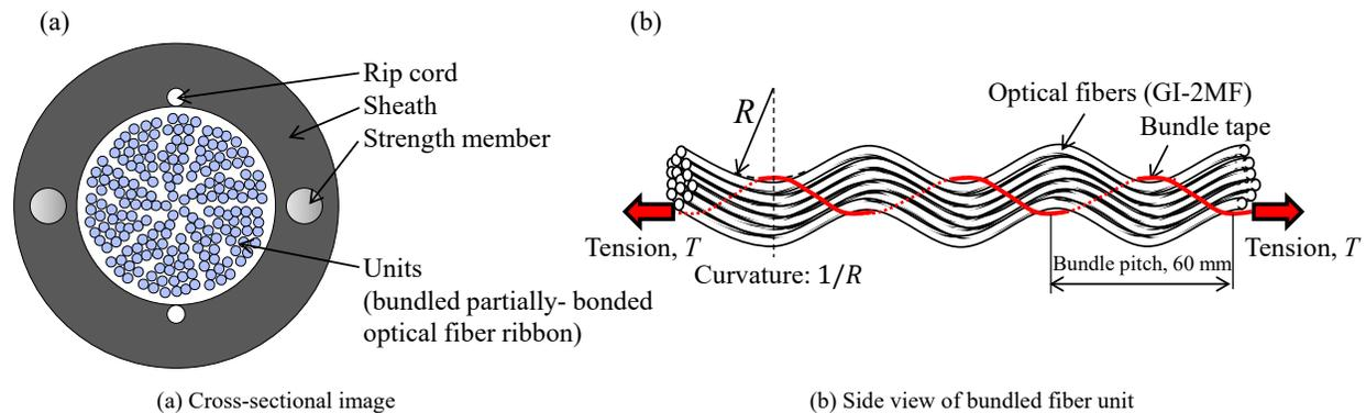
Fig. 3. Schematic image of controlling curvature in high-density cable.
