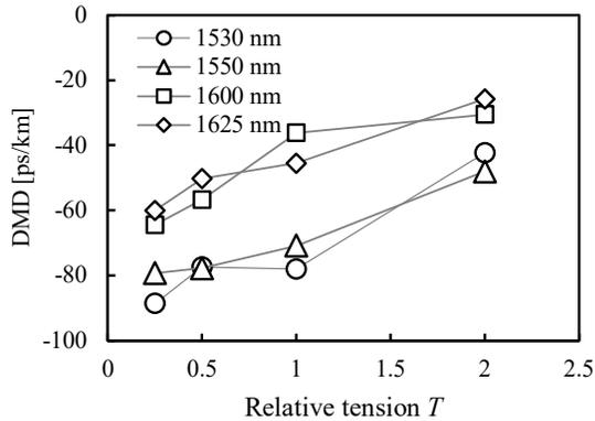
Fig. 4. DMD characteristics as a function of relative tension.
