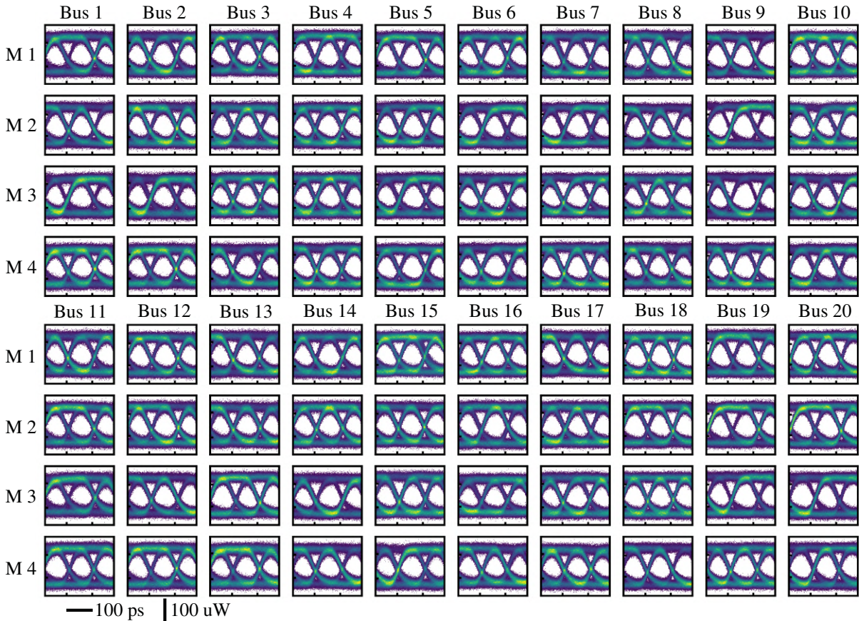
Fig. 2. Eye diagrams from each micro-disk being driven at 10 Gb/s by the 28nm CMOS chip. M 1, 2, 3, 4 correspond to each modulator on the bus.
