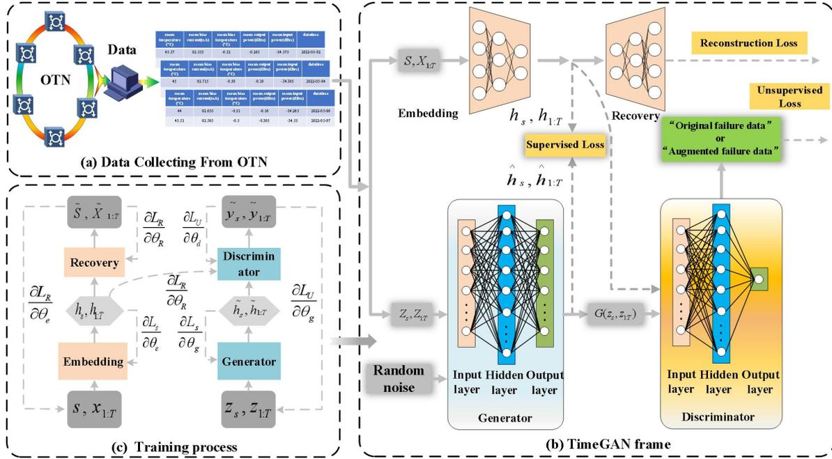
Fig. 1. (a) Data collecting, (b) TimeGAN Frame, (c) Training process. The solid line represents the forward propagation of data, and the dashed line represents the back propagation of gradient and loss.
