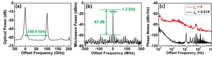
Fig. 3. (a) Optical spectrum and (b) microwave spectrum of the generated sub-THz signal at 101.2 GHz after stabilization when  $(\xi_{12}, f_i) = (0.268, 100.4 \text{ GHz})$  and  $\xi_{21} = 0.015$ . (c) SSB phase noise of the generated sub-THz signal before (red curve) and after (black curve) stabilization.
