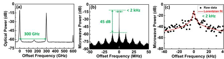
Fig. 4. (a) Optical spectrum (experimental measurement) and (b)(c) microwave spectra (numerical calculation) of the generated sub-THz signal at 300 GHz.
