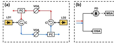
Fig. 1. Schematic diagram of (a) the mutual injection system and (b) the detection system. LD1, laser diode 1; LD2, laser diode 2; FC, fiber coupler; C, circulator; VOA, variable optical attenuator; PD, photodetector; OSA, optical spectrum analyzer; MSA, microwave spectrum analyzer.
