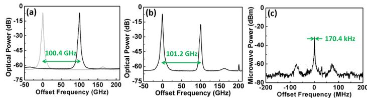
Fig. 2. (a)(b) Optical spectra and (c) microwave spectrum of the P1 dynamics at  $(\xi_{12}, f_i) = (0.268, 100.4 \text{ GHz})$  when  $\xi_{21} = 0$ . The axes in (a) and (b) are relative to 193.28 THz, and the axis in (c) is relative to 101.2 GHz.
