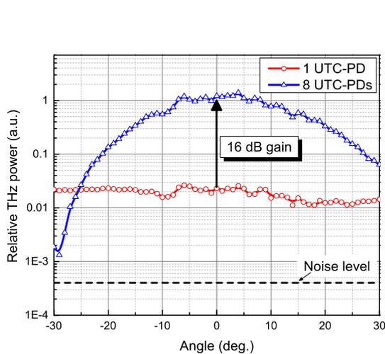
Fig. 4: Radiation pattern of 300-GHz beam combining by aligned optical phase.
