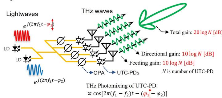
Fig. 1: Schematic of optoelectronic THz beam steering with large-scale planar photonic integration technology.
