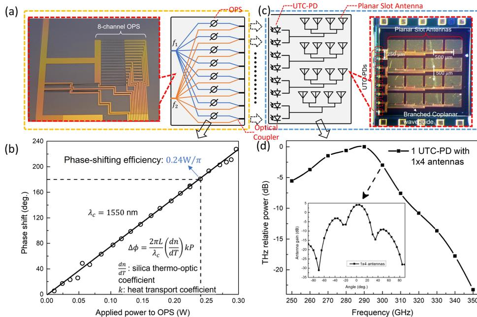
Fig. 2: (a) Schematic and photograph of 8-channel OPA. (b) The OPS phase shift characteristic at 1550 nm. (c) Layout and photo of 8 arrayed UTC-PDs with integrated  $4 \times 4$  PSA array. (d) Frequency dependency of  $1 \times 4$  antennas with an excited UTC-PD. The inset is simulated 300-GHz beam pattern.
