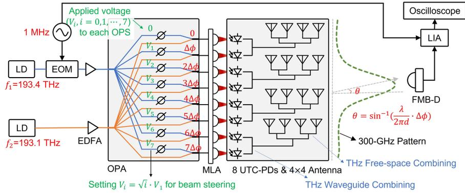
Fig. 3: Experiment setup for 300-GHz beam combining and steering.
