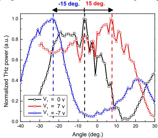
Fig. 5: Radiation pattern of 300-GHz beam steering by gradient optical phase.  $V_1$  is the applied voltage to the OPS of channel 1 and the other applied voltages satisfy  $V_i = \sqrt{i} \cdot V_1$  ( $i$  is the channel number).
