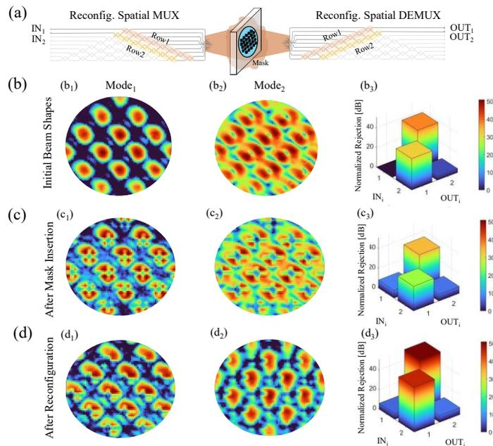
Figure 3. (a) Schematic of the setup for performing (de)multiplexing (b) initial beams shapes and mode rejection automatically obtained before inserting the mask, (c) same after insertion of the mask, (d) the new beam shapes and mutual rejection obtained after reconfiguration.
