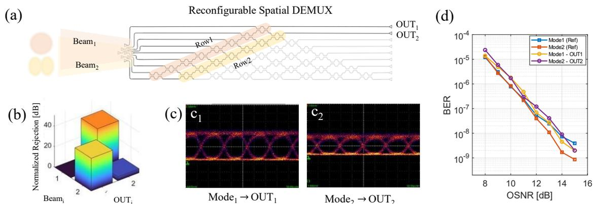
Figure 2. (a) Demultiplexing two orthogonal beams using meshes of MZI, (b) Normalized mode rejection for the extracted beams, (c) Eye diagrams for the 10 Gbit/s received signals at OUT1 (c<sub>1</sub>) and OUT2 (c<sub>2</sub>), (d) BER measurements for established channels
