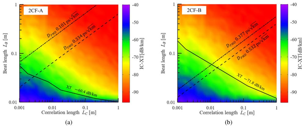
Fig. 2. Plot of the simulated and measured IC-XT and  $D_{PMD}$  of: (a) 2CF-A and (b) 2CF-B .
