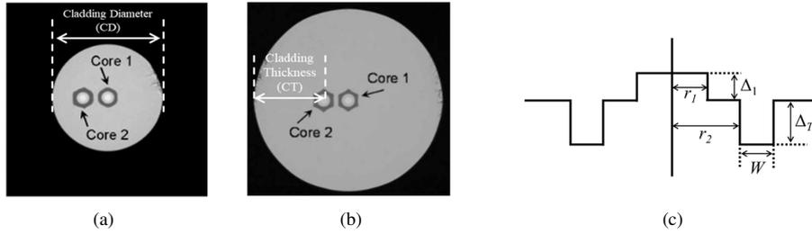
Fig. 1. Cross-section views of fibers (a) 2CF-A and (b) 2CF-B, and (c) core refractive index profile [3].
