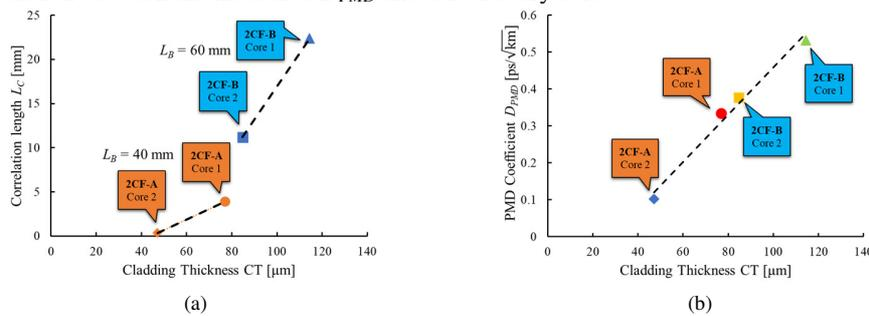
Fig. 3. (a) Relation between  $L_C$  and CT, and (b) between  $D_{PMD}$  and CT of every core in 2CF-A and 2CF-B.
