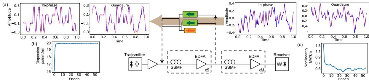
Fig. 3 (a) Backward NLSE operator for 5 spans (0.2StPS) along with 32 symbols of the received and transmitted signals, and the sampling rate is 4 samples per symbol. The optimization of (b) dispersion and (c) nonlinear index in the zero-attenuation 5-span backward NLSE.
