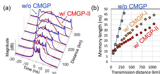
Fig. 5. (a): Evolutions of impulse response in 10-mode transmission. (b): Memory length growth along distance.
