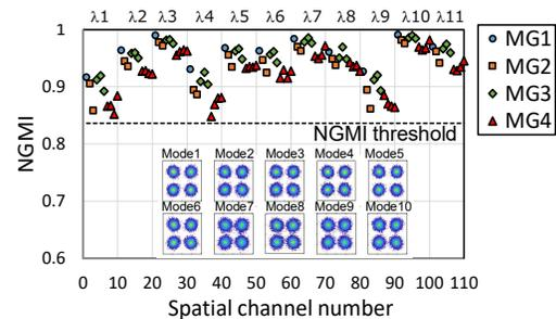
Fig. 7. NGMI for all channels after 10-spatial-mode 1300-km transmission. Inset shows representative constellations of wavelength channel #7.
