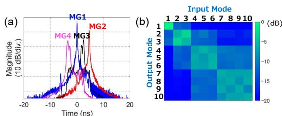
Fig. 4. (a): Impulse response for each MG at 52 km. (b): Intra/inter-mode crosstalk matrix at 52 km.
