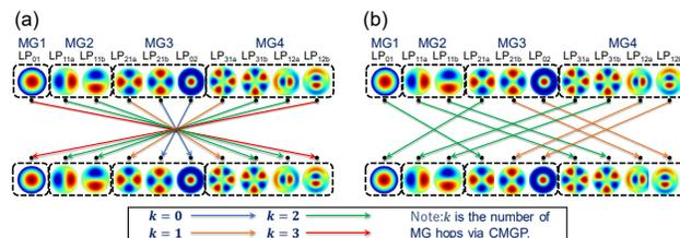
Fig. 2. Inter-connection options in CMGP. (a) CMGP-I (symmetric interchange) and (b): CMGP-II (forced interchange).
