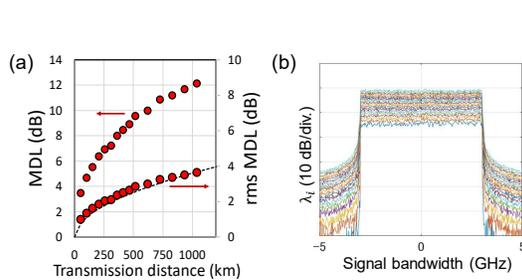
Fig. 6. (a): Accumulation of peak-to-peak MDL and rms MDL along transmission distance. (b): Eigenvalue distribution for all spatial channels at 1300 km.
