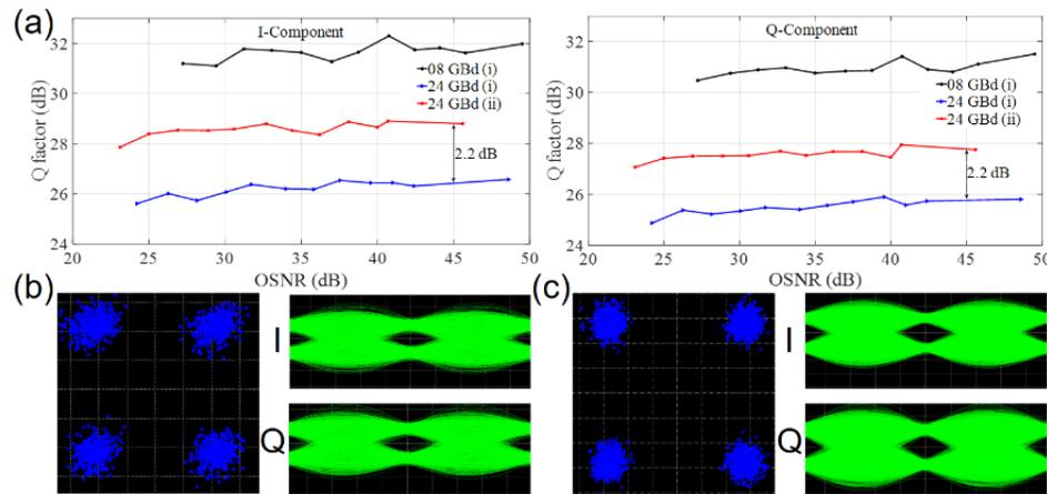
Fig. 3 (a) I and Q component of the Q-factor measurements for the detection of a 12 GHz signal in a 12 GHz bandwidth (blue), a 4 GHz signal in a 4 GHz bandwidth (black) and a 12 GHz signal in a 4 GHz bandwidth with the proposed method (red). The constellation and eye diagrams for direct measurement (b) and the proposed method (c).
