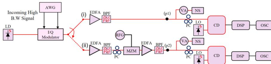
Fig. 2 Experimental setup for comparing the direct measurement (i), and the proposed method (ii). LD: laser diode, AWG: arbitrary waveform generator, EDFA: erbium-doped fiber amplifier, BPF: bandpass filter, PC: polarizer controller, MZM: Mach-Zehnder modulator, VA: variable attenuator, NS: noise source, LO: local oscillator, CD: coherent detector, DSP: digital signal processing, OSC: oscilloscope.
