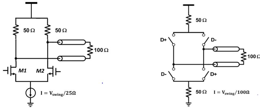
Fig. 4. CML (left) and SST (right) driver output stage
