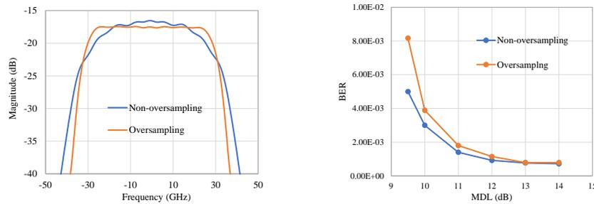
Fig. 2. Comparison of signal spectrum and BER performance between RRC pulse shaping using x1.2 DAC sampling ratio and non-oversampling.
