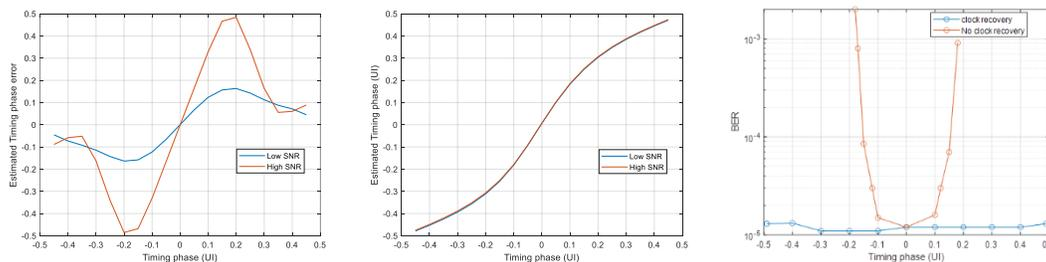
Fig. 5. Mull-Muller (left), Cisco (middle), Ber vs clock phase error (right)
