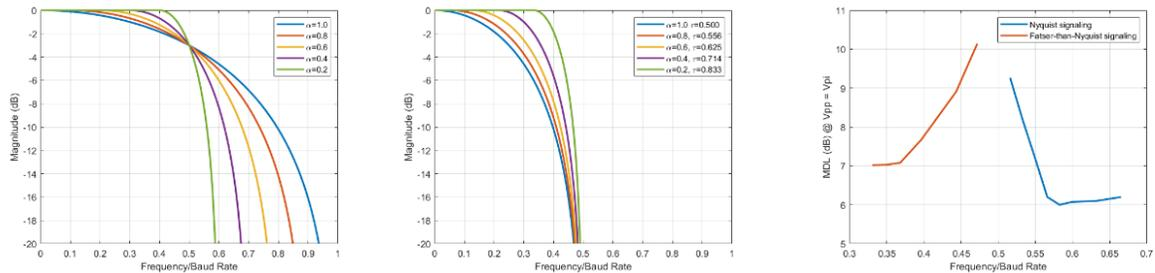
Fig. 3. Nyquist signaling (left) and Fast-than-Nyquist signaling (middle) with the same RRC pulse shaping function  $h(t)$  at different excess-bandwidth factor  $\alpha$ . FTN signaling has a time acceleration factor  $\tau = \frac{1}{1+\alpha}$  such that the signal spectrum is limited within the Nyquist frequency (i.e., 1/2 baud rate). Nyquist signaling and FTN have different MDL vs. 6-dB BW characteristics (right).
