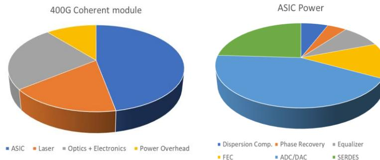
Fig. 1. Power breakdown of 400G ZR coherent transceiver
