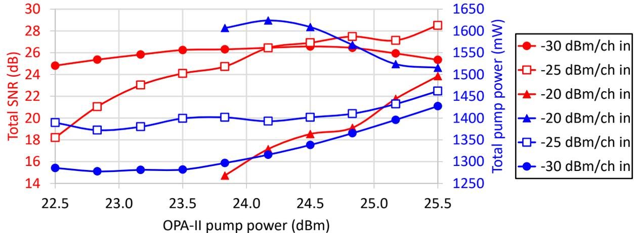
Fig. 3. Total SNR (red, left scale) and total pump power (blue, right scale) for three input power levels (filled circles for  $-30$  dBm/ch, empty squares for  $-25$  dBm/ch, filled triangles for  $-20$  dBm/ch) vs. the OPA-II pump power at fixed 20 dB total gain.
