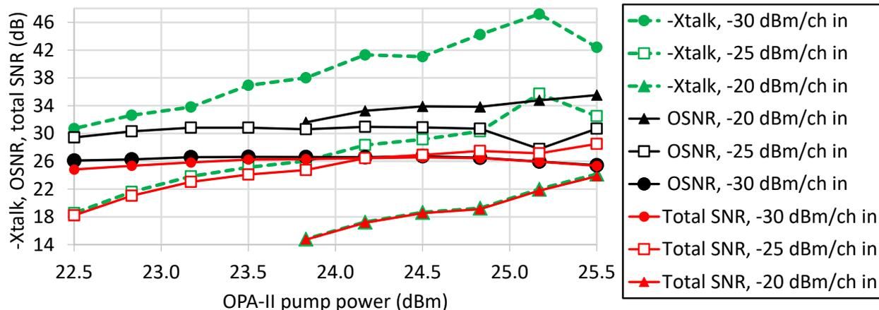
Fig. 2. Inverse FWM crosstalk ( $-Xtalk$ , green), OSNR (black), and total SNR (red) for three input power levels (filled circles for  $-30$  dBm/ch, empty squares for  $-25$  dBm/ch, filled triangles for  $-20$  dBm/ch) vs. the OPA-II pump power at fixed 20 dB total gain.
