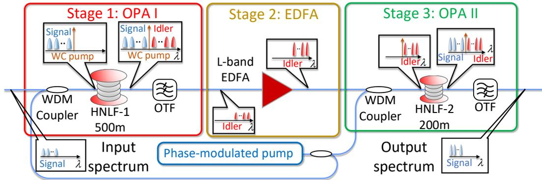
Fig. 1. Schematic of the hybrid S-band amplifier. EDFA: erbium-doped fiber amplifier; HNLF: highly-nonlinear fiber; OPA: optical parametric amplifier; OTF: optical tunable filter; WC: wavelength conversion; WDM: wavelength-division-multiplexer.
