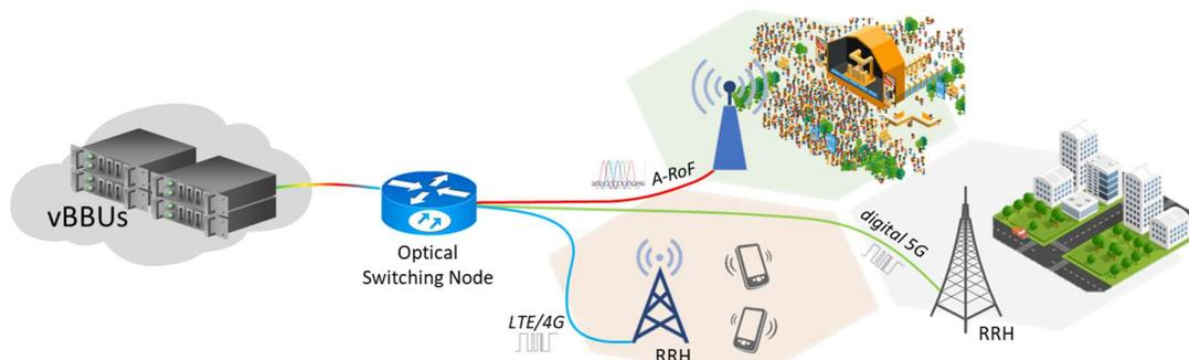
Fig. 1 A WSS-based hybrid optical transport architecture
