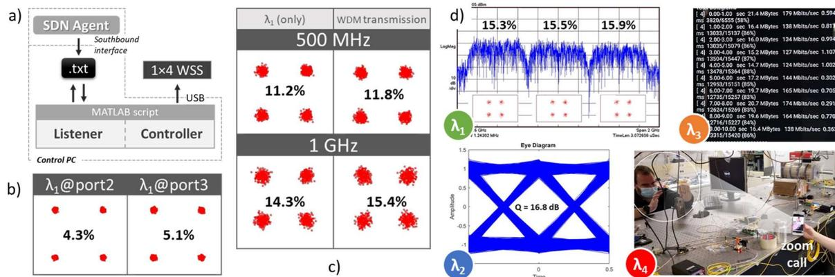
Fig. 3: (a) The SDN interface script for the WSS control, (b) Constellation diagrams corresponding to switching of  $\lambda_1$  between port 2 and port 3 of WSS, (c) Performance evaluation of  $\lambda_1$  after single and WDM transmission, (d) Evaluation of successful concurrent 4 $\lambda$  transmission.
