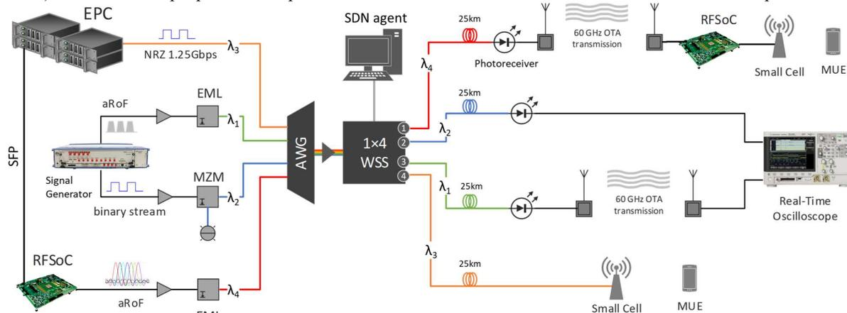
Fig. 2: The 4 $\lambda$ -optical transport experimental layout
