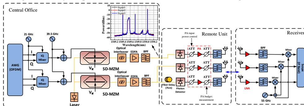
Fig. 1. Experimental setup of 3×3 MIMO V-band RoF system
