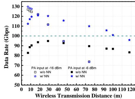
Fig. 5. Maximum data rate over different transmission distances
