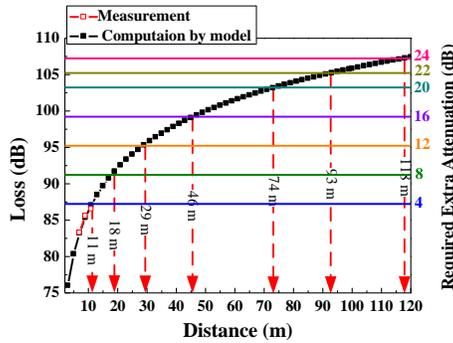
Fig. 4. Experimental and model results for 60 GHz path loss
