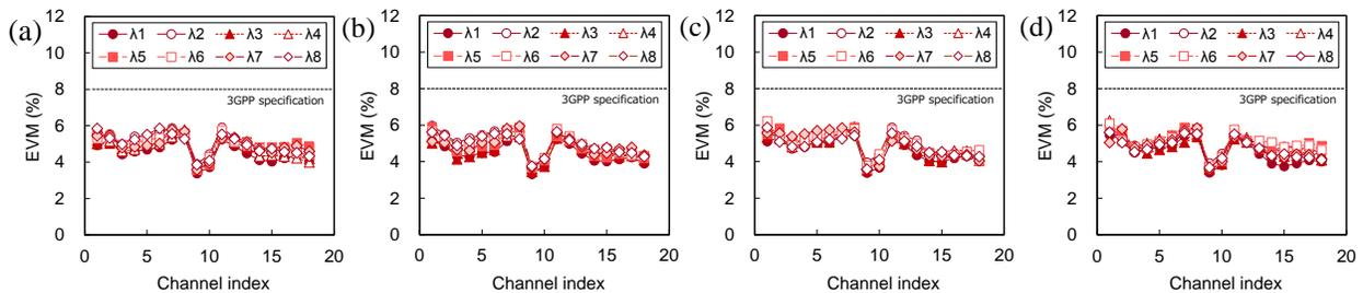
Fig. 5. Measured EVM values after the 12.8-km MCF transmission (a) on the first core, (b) on the second core, (c) on the third core, and (d) on the fourth core.
