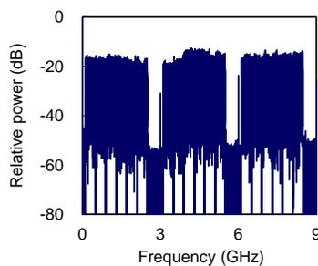
Fig. 2. RF spectrum before the LN-MZM.
