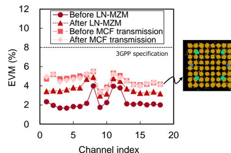
Fig. 4. EVM values for the first wavelength on the first core.
