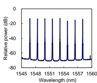
Fig. 3. Optical spectrum before the FI.
