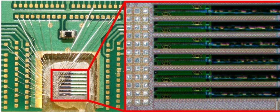
Fig. 2 Assembled and wirebonded device on PCB with closeup of PIC. Chip footprint is dominated by edge couplers
