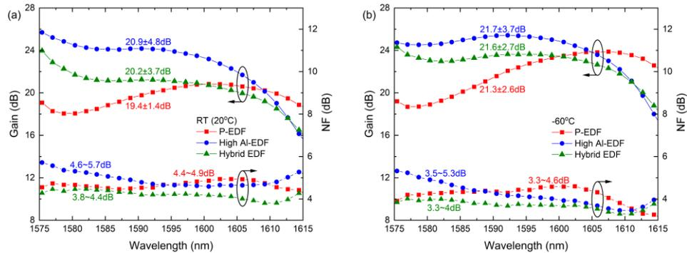
Fig. 2. (a) Gain and NF spectra at RT (20°C) and (b) -60°C for 30m of P-EDF, 15m of high Al-EDF, and hybrid EDF comprising 15m of P-EDF and 5.5m of high Al-EDF. The total pump power launched into the EDFs was 765mW.
