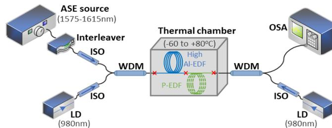
Fig. 1. Schematic of the experimental setup for the L-band EDFA.
