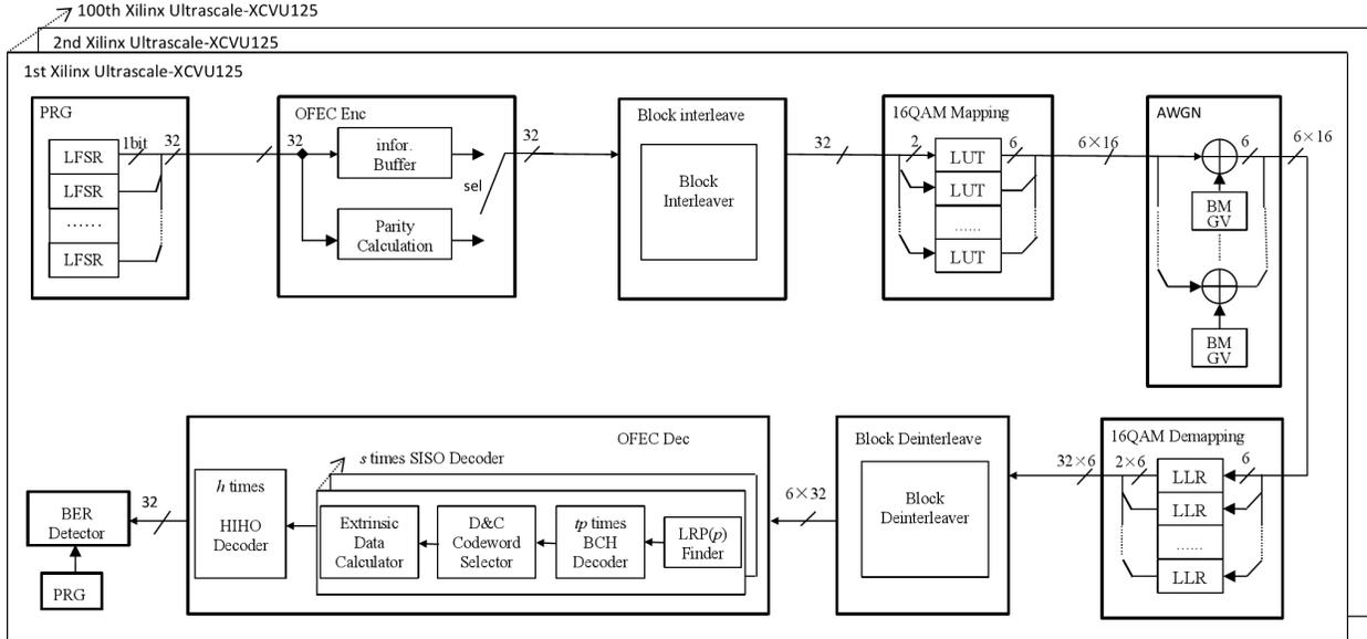
Figure 1: FPGA implementation of the OFEC verification system
