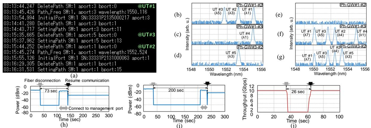
Fig. 3: Experimental results (a) Event log during restoration procedure, (b),(c),(d) Optical spectra before reconfiguration, (e),(f),(g) Optical spectra after reconfiguration, (h) Received power of HDMI signal, (i) Received power of CPRI signal, (j) Throughput of Ethernet signal
