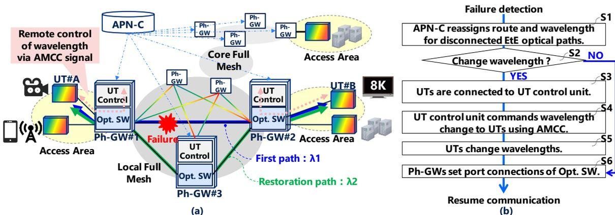
Fig. 1: (a) Restoration architecture in All-Photonics Network, (b) Proposed procedure for EtE optical-path restoration.
