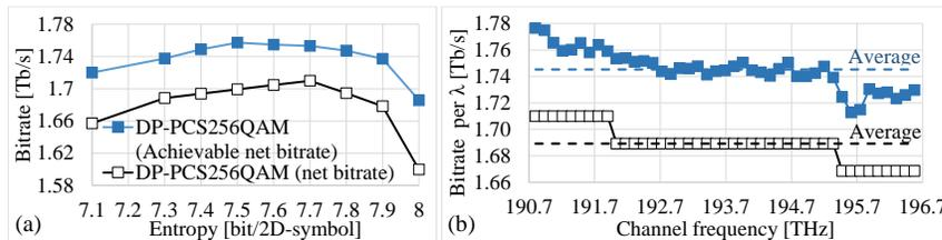
Fig. 3. Bitrate vs entropy (a), bitrate per DWDM channel (b).
