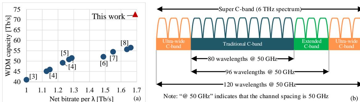
Fig. 1. Reported DWDM capacity vs per-carrier net bitrate exceeding 1 Tb/s/ $\lambda$  (a). Super C-band representation (b).
