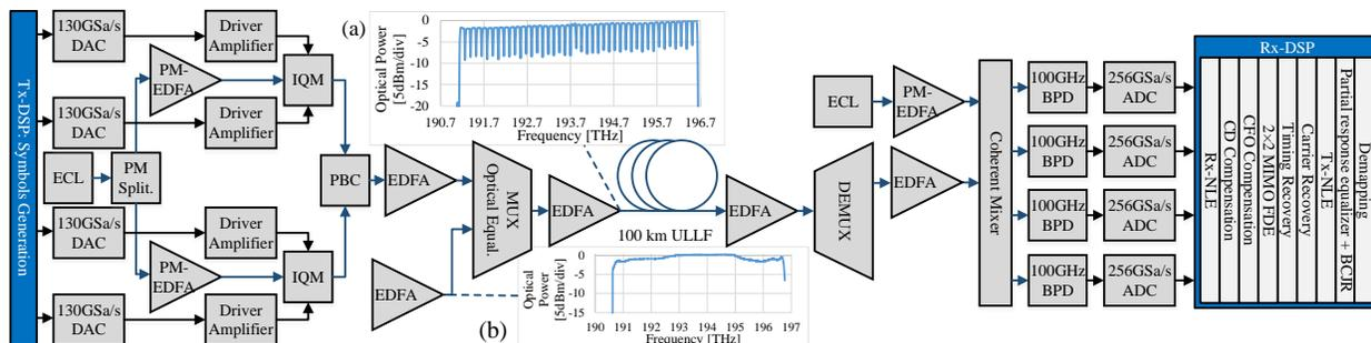
Fig. 2. Schematic of the experimental setup, insets: 43-channel DWDM transmitted spectrum (a) and super C-band EDFA gain spectrum (b).
