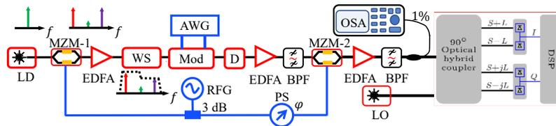
Fig. 2. Proof-of-concept experimental set up for all-optical aggregation. LD: laser diode, MZM: Mach-Zehnder modulator, D: dispersion unit, WS: waveshaper, OSA: optical spectrum analyzer.
