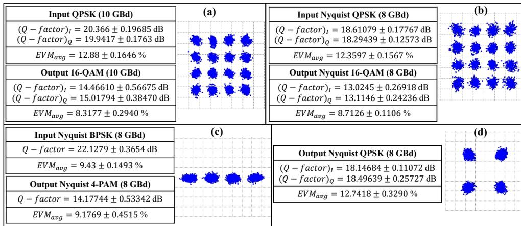
Fig. 3. Measured constellation maps of the aggregated signals along with the  $Q$ -factors and average error vector magnitudes of input and aggregated channels.
