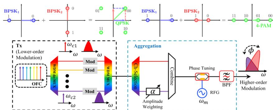
Fig. 1. Principle of vector summation of symbols and the concept of the all-optical aggregation method using electro-optic modulators. OFC: Optical frequency comb, Mod: modulator, BPF: bandpass filter, RFG:
