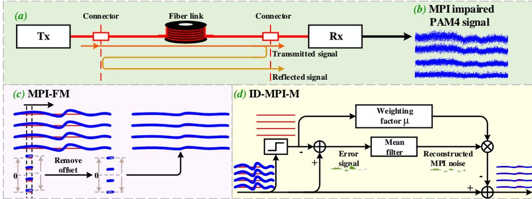
Fig. 1. (a) The schematic diagram of the MPI noise generation, (b) the simulated MPI impaired PAM4 signal, (c-d) the schematic diagram of the proposed two MPI mitigation algorithms.
