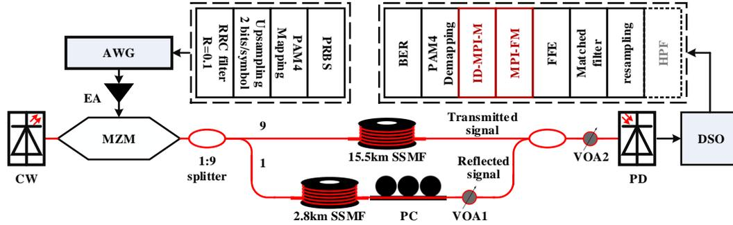
Fig. 2. Experimental setup of the MPI impaired IMDD PAM4 system.
