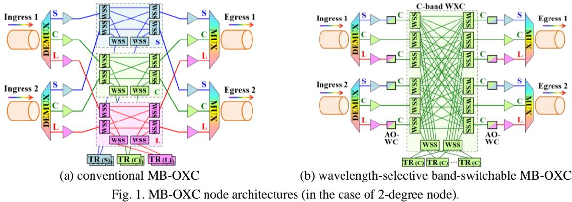
Fig. 1. MB-OXC node architectures (in the case of 2-degree node).
