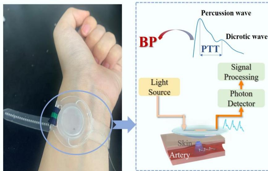
Fig. 2. The schematic of the continuous blood pressure monitoring smartwatch based on optical fiber.
