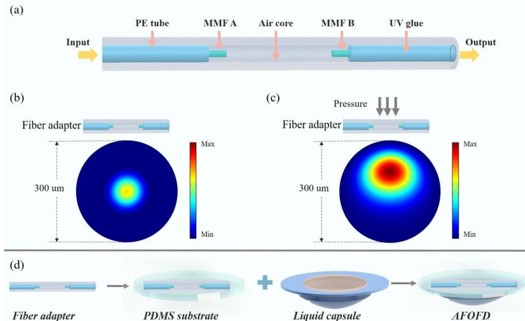
Fig. 1. (a) The structure of the fiber adapter. (b) Optical field energy density distribution of the straight optical fiber adapter. (c) Optical field energy density distribution of the pressed optical fiber adapter. (d) The fabrication of alignment-free optical fiber-based device.
