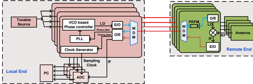
Fig. 1. The principle of the proposed distributed receiving system.
