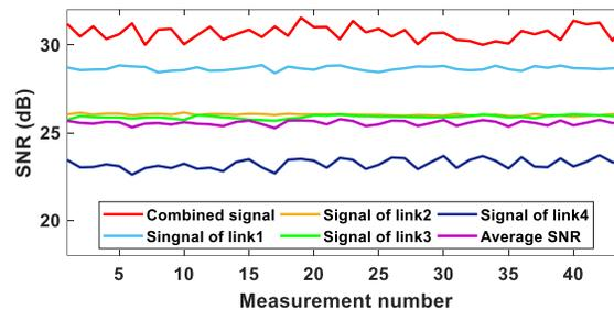
Fig. 4. The SNRs of each received signal and the combined signal.
