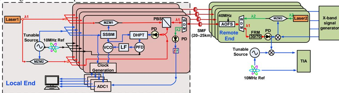
Fig. 2. The experimental setup of the proposed distributed receiving system.
