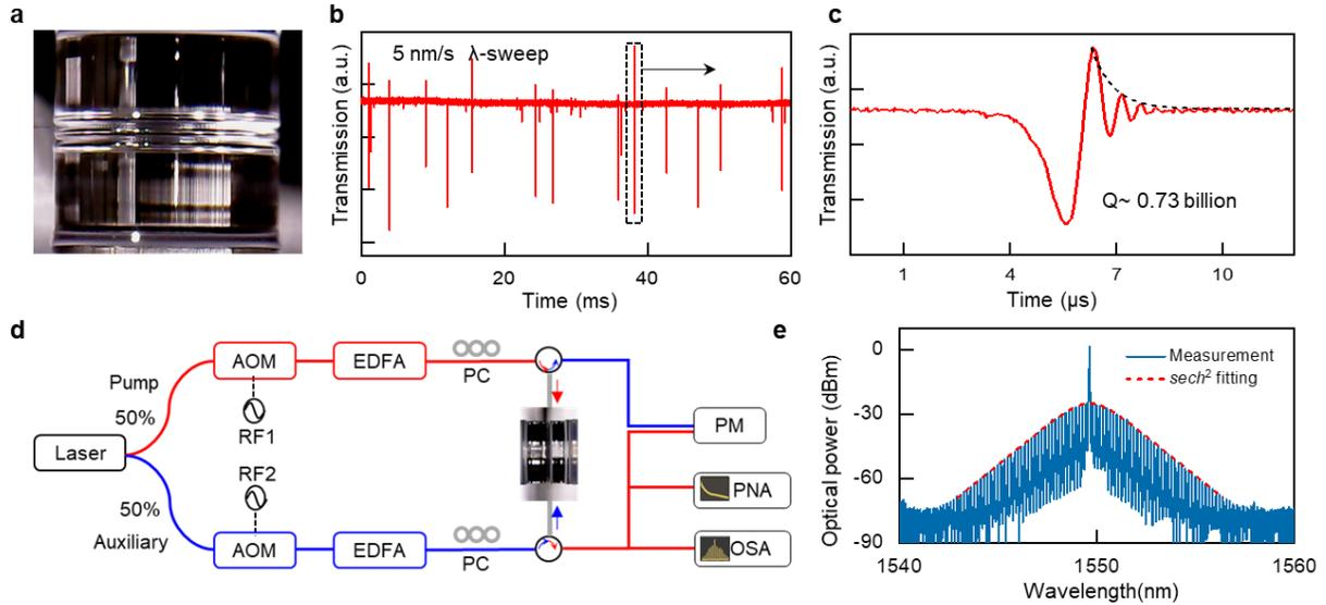
Fig. 1. a. WGM micro-rod picture. b. micro-cavity transmission and c. Ring down measurement of the pump cavity mode. d. Experimental setup. e. Generated soliton microcomb spectrum.
