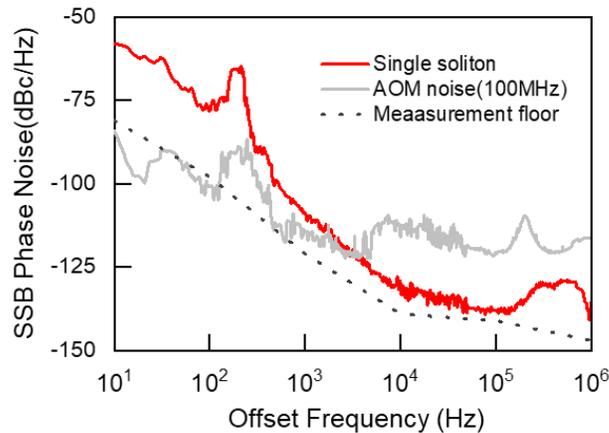
Fig. 2. SSB phase noise of the 21.5 GHz microwave generated by photo-detecting  $\nu_{\text{rep}}$ .
