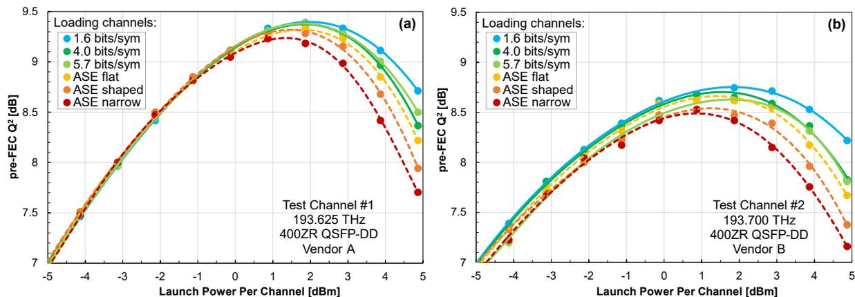
Fig. 2. Pre-FEC  $Q^2$  for both test channels with different bandwidth loading of 2.4 THz WDM spectrum over 24 dB TW-RS fiber link.
