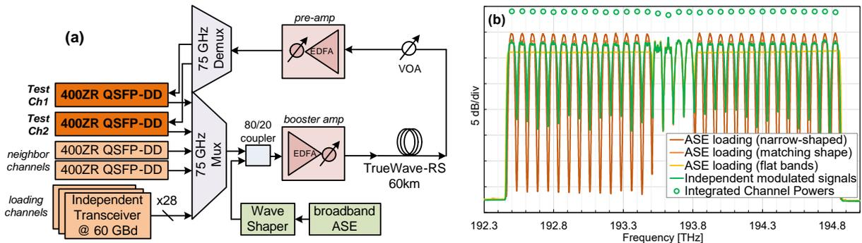
Fig. 1. (a) Experimental configuration and (b) measured optical spectrum at booster amplifier output with a resolution bandwidth of 0.02 nm.
