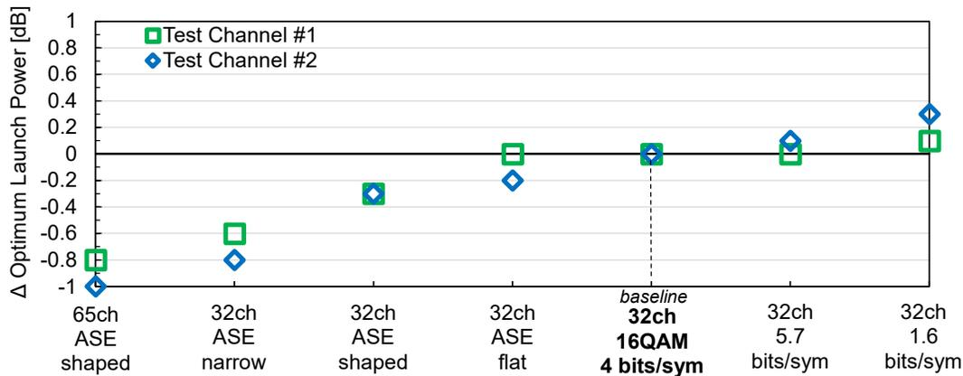
Fig. 3. Relative change in optimum launch power for different bandwidth loading conditions on 24 dB TW-RS link.
