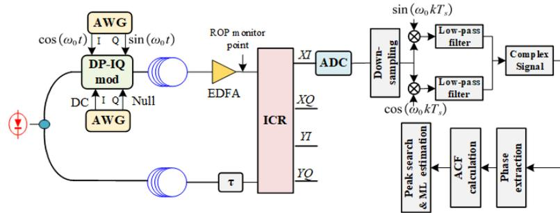
Figure. 1 Simulation setup and DSP offline of CPA estimation method by using SHC system
