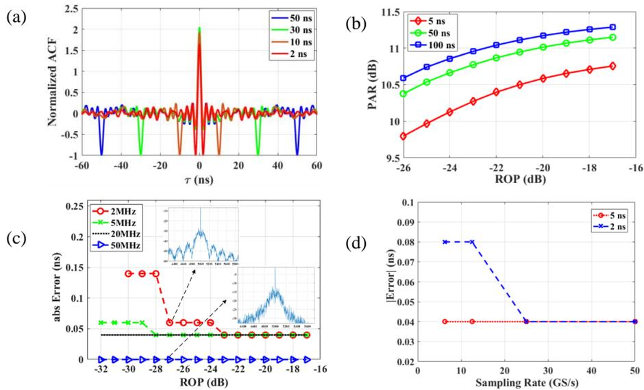
Figure. 2 (a) The normalized ACF versus delay time without low-pass filter (b) the PAR function of ROP (c) the error versus ROP, under different linewidths and delay time (d) The error function of sampling rate at 45MHz of laser.
