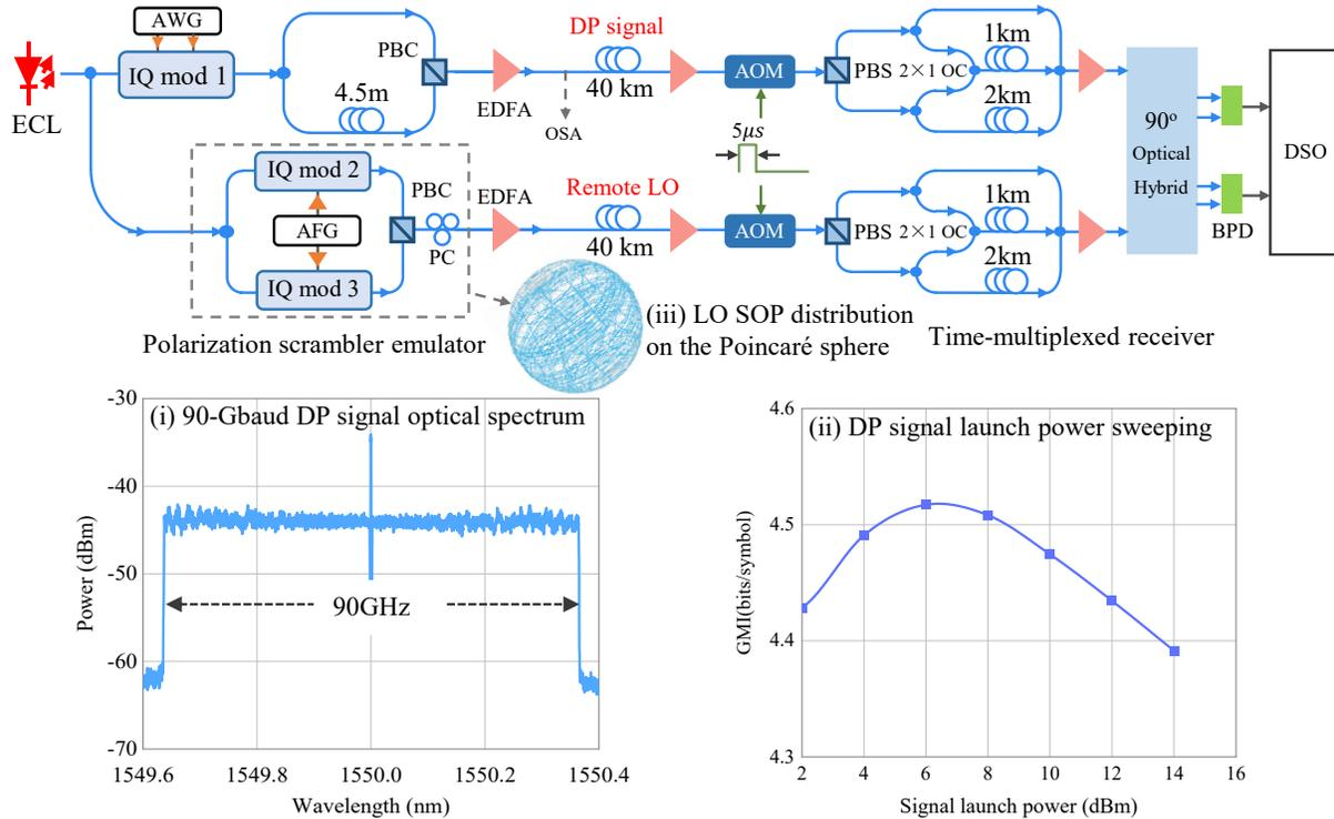
Fig. 2: Experimental setup for C-PDCR. ECL: external cavity laser. IQ mod: IQ modulator. AWG/AFG: arbitrary waveform/function generator. PC: polarization controller. PBS/PBC: polarization beam splitter/combiner. EDFA: Erbium-doped fiber amplifier. OSA: optical spectrum analyzer. AOM: acoustic-optic modulator. DSO: digital sampling oscilloscope.
