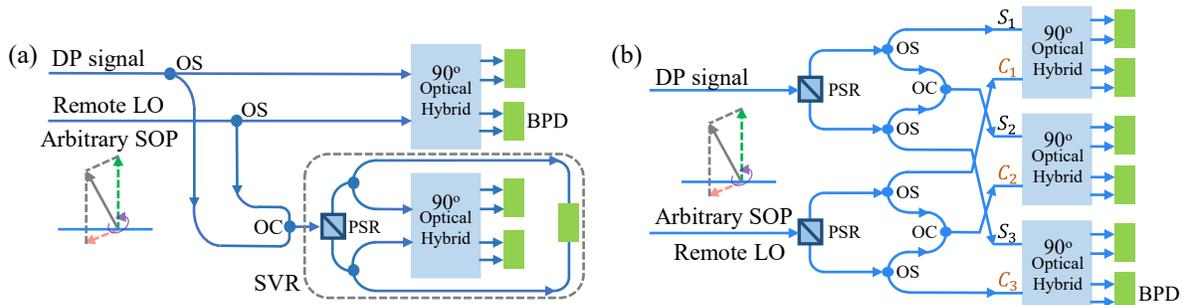
Fig. 1: Schematic of proposed (a) H-PDCR and (b) C-PDCR without any optical polarization control for remotely delivered LO. PSR: polarization splitter/rotator. OC/OS: optical coupler/splitter. SVR: Stokes vector receiver. BPD: balanced photodetector. PoL: polarization. SOP: state of polarization.
