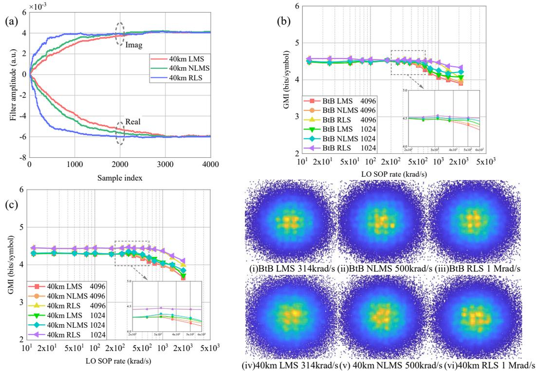
Fig. 3: (a) Convergence rate comparison between different algorithms by observing filter coefficients. GMI performance as a function of LO SOP rotation speed at BtB (b) and 40 km (c) under 25-dB OSNR by using different algorithms with coefficients updated after a different number of symbols for MIMO. Insets show the recovered PCS 256-QAM constellations with coefficients updated once every 4096 symbols.
