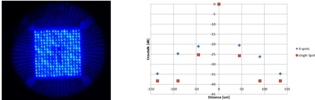
Fig. 2. 16x16 array of 4 $\mu$ m diameter emitters, with 30 $\mu$ m spacing as seen through a 1mm plastic imaging fiber. DC cross-talk was measured from 4 illuminated spots to an adjacent detector and from a single illuminated emitter to other detector.
