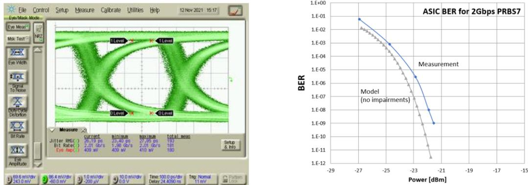
Fig. 3. Received electrical eye and waterfall chart showing link with integrated PD/TIA made in 130nm process. Total power consumption including driver and receiver, (not including the 50 Ohm drive) was <2pJ/bit.
