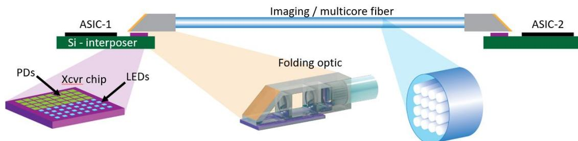
Fig. 1. Concept: The transceiver chip translates electrical data from the ASIC to a wide optical bus with a large array of light emitters and receives signals with an integrated photodetector/TIA array. A large number of beams are carried by a multi-core or imaging fiber through an optional folding optic.
