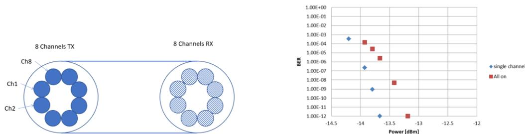
Fig. 3. 8 channel emitter array and photodetector array used to measure crosstalk. 8 commercial TIAs received the signals simultaneously the impairment measured with all channels on.
