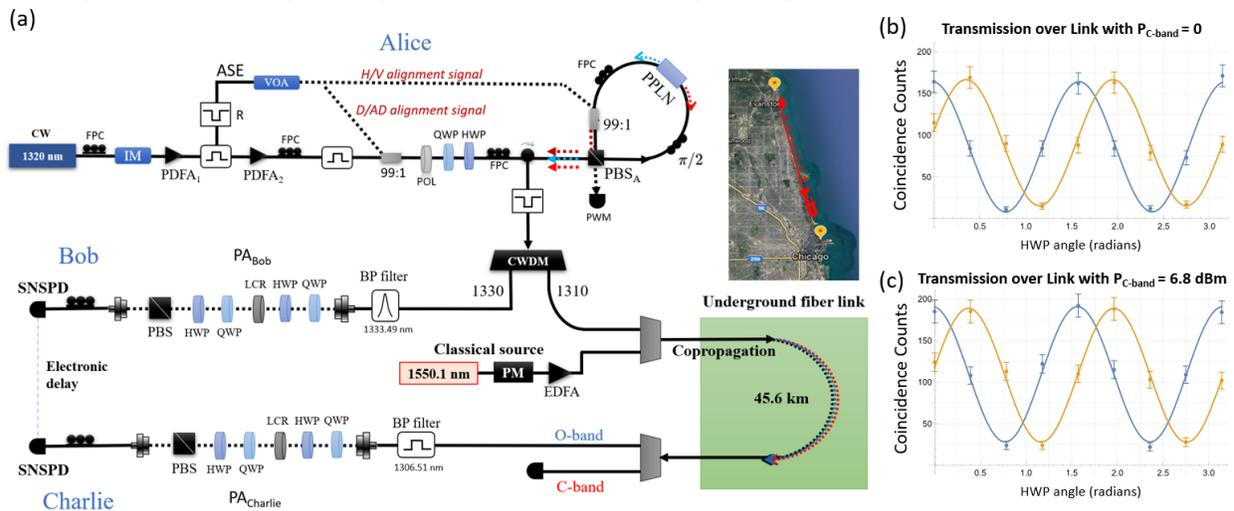
Fig. 1: (a) Experimental diagram for polarization entanglement source with built-in basis alignment signal and entanglement distribution over underground fiber link in the presence of C-band classical light. (b) and (c) TPI measurements: (b) Entangled photon sent over distribution fiber without classical light. (c) Entangled photon sent over distribution fiber with 6.8 dBm of copropagating classical light.
