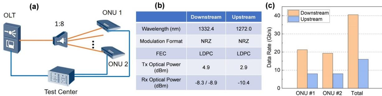
Fig. 1. (a) Experimental setup for the characterization of the real-time 50G TDM-PON, (b) optical parameters of the 50G PON prototype in both downstream and upstream transmission, (c) measured results of data throughputs of two ONUs for both downstream and upstream.
