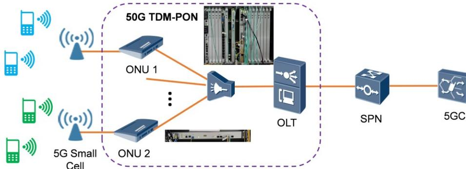
Fig. 2. Schematic setup of the field trial of 50G PON based small cell backhaul.
