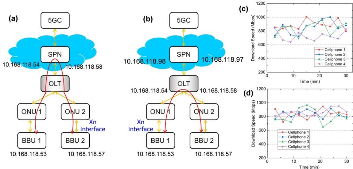
Fig. 3. The network structure for the 50G PON based small cell backhaul accompanied with IP addresses of each equipment when OLT configured at (a) L2 and (b) L3, and the measured download speed of each UEs using (c) L2 and (d) L3 PON networking.
