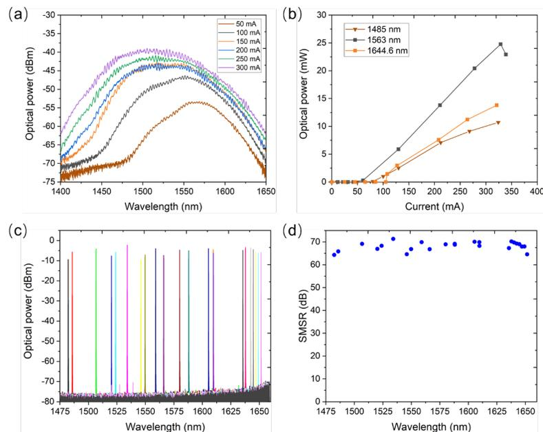
Fig. 2. (a) Measured ASE spectra of the RSOA. The ripple is below 0.5 dB. (b) Measured L-I curves at several typical wavelengths. The maximum power is 24.8 mW under a 329 mA pump current. (c) Superimposed lasing spectra of the hybrid-integrated laser. The wavelength tuning range is about 170 nm. (d) Extracted SMSR as a function of lasing wavelength. The SMSR exceeds 64 dB in the entire wavelength tuning range.
