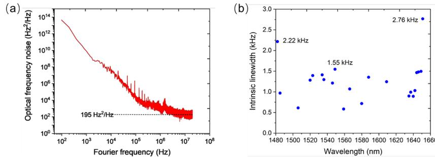
Fig. 3. (a) OFN power spectral density at the lasing wavelength of 1506 nm. The output power is 7.8 dBm at an injection current of 300 mA. (b) Intrinsic linewidth measured at various wavelengths.
