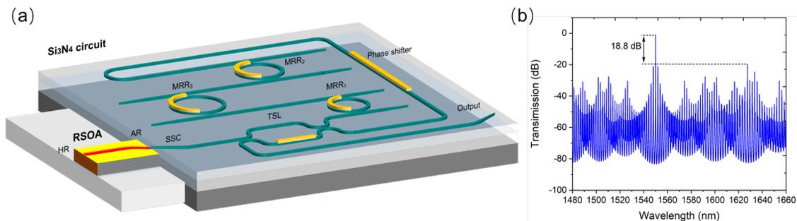
Fig. 1. (a) Schematic structure of the hybrid-integrated external cavity laser. HR, high-reflection coating; AR, anti-reflection coating; SSC, spot-size converter; MRR, microring resonator; TSL, tunable Sagnac loop. (b) Simulated transmission spectrum of the Vernier filter. The passive side mode suppression ratio is 18.8 dB.
