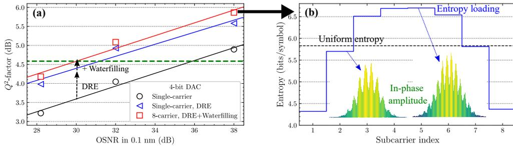
Fig. 4. (a)  $Q^2$ -factor versus OSNR using a 4-bit DAC, showing the benefits of DRE and waterfilling; (b) Entropy loading values mapped to subcarriers at highest OSNR.
