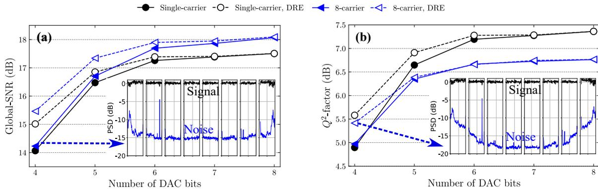
Fig. 2. (a) Global-SNR and (b)  $Q^2$ -factor versus the number of DAC bits, without and with DRE.
