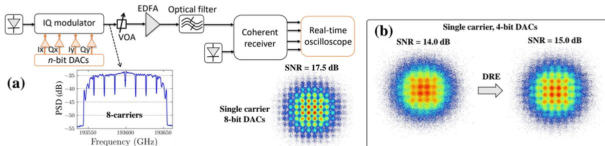
Fig. 1. (a) Experimental setup, insets show an example 8-carrier spectrum and PCS-256QAM constellation using 8-bit DAC; (b) Constellations using 4-bit DAC without and with DRE.
