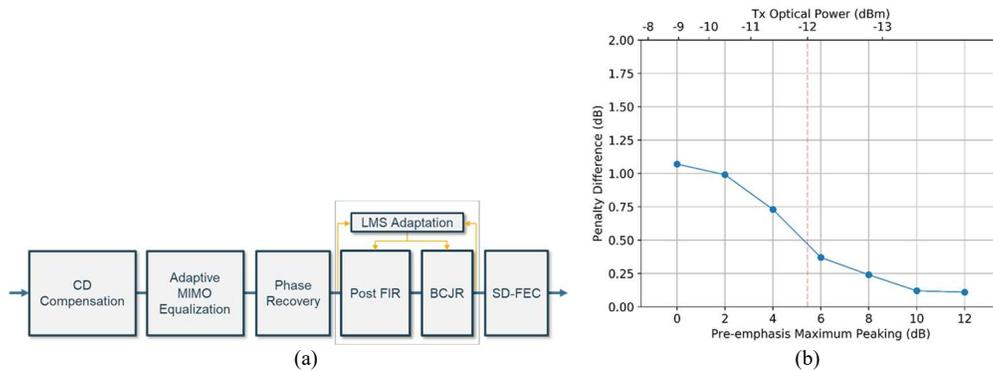
Fig. 3 (a) Block diagram of coherent receiver DSP with partial response equalizer block consisting of a post FIR noise-whitening filter and a MAP detector, and (b) simulated sensitivity difference between pre-emphasis filter and partial response filter with realistic transmitter and receiver model for 800G QAM16 at pre-FEC BER threshold of  $2.2 \times 10^{-2}$ . Note that partial response filter can have as much as 0.45 dB sensitivity improvement at -12 dBm of Tx transmit power.
