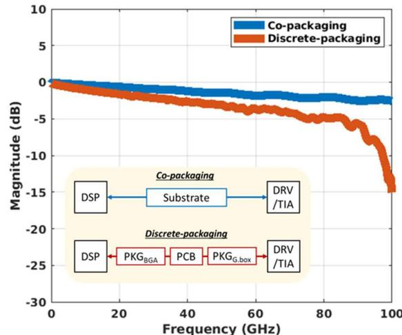
Fig. 1. Exemplary simulated frequency response of die-to-die RF connection between DSP and DRV/TIA for co-packaging and discrete-packaging options, respectively.
