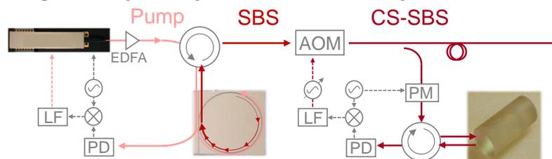
Figure 1. Cavity-stabilized stimulated Brillouin scattering (CS-SBS) laser [6]. An amplified narrow linewidth semiconductor laser [9] is used to pump an integrated SBS laser. An acousto-optic modulator is used to stabilize the SBS laser using a 1 Billion Q optical reference cavity [10].
