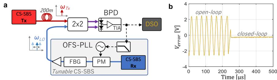
Figure 3. a) Two cavity-stabilized SBS lasers (CS-SBS) are employed in the optical-frequency-stabilized phase locked loop (OFS-PLL) [6]. A balanced detector (BPD) with transimpedance amplifier (TIA) is an optical phase detector. Phase modulator (PM), fiber Bragg grating (FBG) realize a tunable sideband as local oscillator. b) phase error sampled by digital storage oscilloscope (DSO) in open- and closed-loop operation
