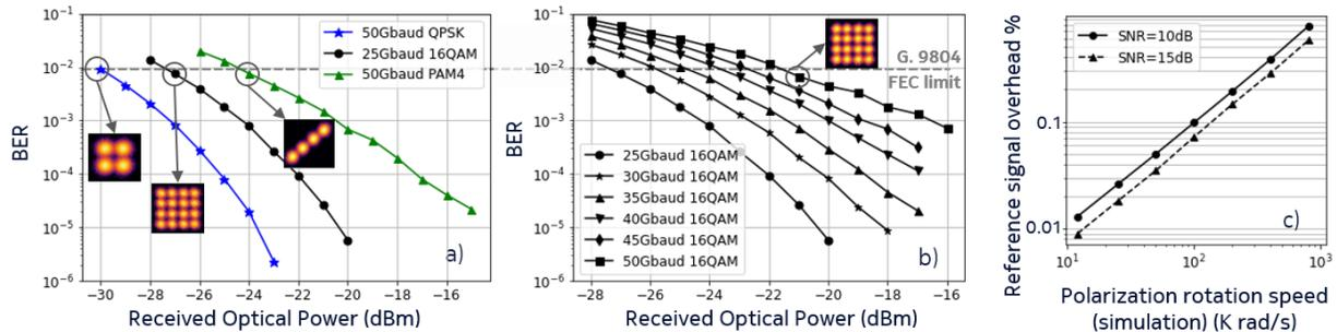
Fig. 3 a) Performance comparison of 100 Gb/s PAM4/QPSK/16QAM signals; b) BER performances of 16QAM signal with different baud rates up to 50 Gbaud/s; c) Minimum required reference signal overhead for  $W_{adaptive}$  training (simulation of 50Gbaud 16QAM).
