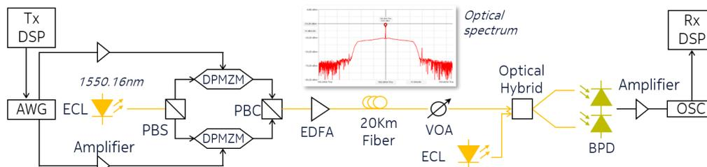
Fig. 2 Experimental setup (inset shows optical spectrum of a 50 Gbaud 16QAM signal). PBS: polarization beam splitter; DPMZMs: dual-parallel Mach-Zehnder modulators; PBC: polarization beam combiner.
