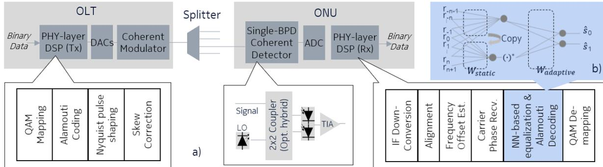
Fig. 1. a) A polarization-insensitive coherent PON system (downstream only) with the single-BPD-based receiver and b) the multi-purpose neural network in the receiver DSP, in which (·)\* means conjugation
