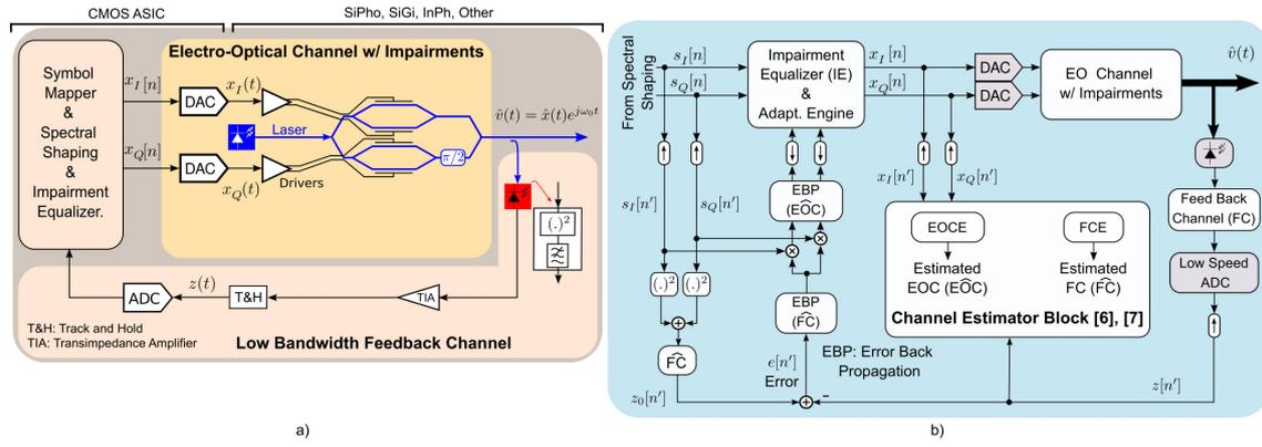
Fig. 1: Coherent optical transmitter with an all-digital adaptive background compensation system based on a low bandwidth feedback channel. a) Top view of the proposed architecture. b) Block diagram of the compensation system for one polarization. Ideal PD, DACs, and ADC stages are assumed (bandwidth limitations and impairments are included in both EO channel (EOC) and feedback channel (FC) blocks).
