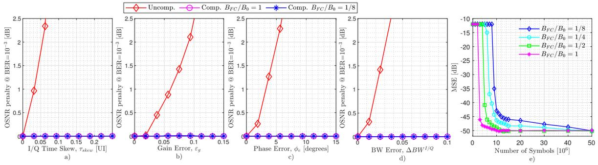
Fig. 2: OSNR penalty versus (a) Tx I/Q time skew, (b) gain error, (c) phase error, and (d) bandwidth error, at BER = 10<sup>-3</sup> for a feedback channel with  $B_{FC} = B_0$  and  $B_{FC} = B_0/8$ . (e) MSE vs different feedback bandwidths,  $B_{FC}$ .
