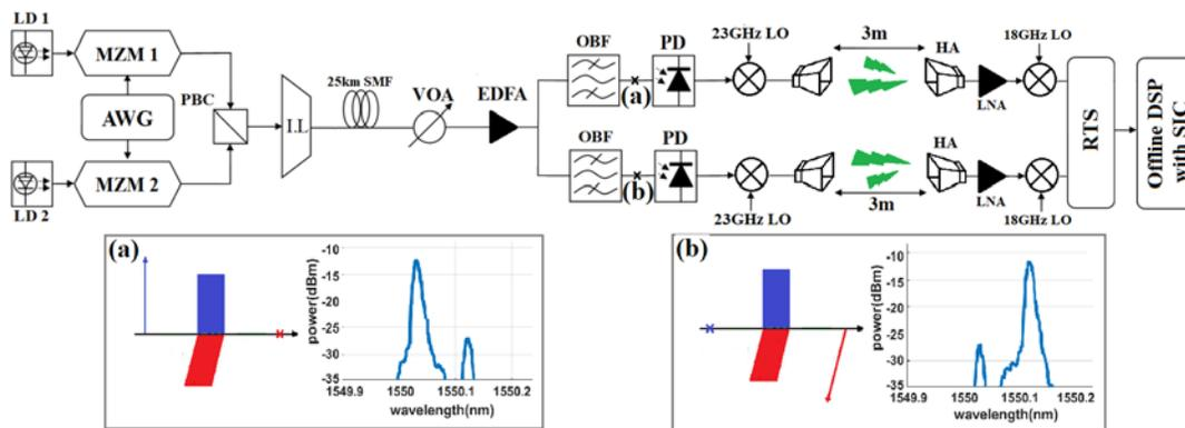
Fig. 2. The experiment setup and spectra of (a) *x*-polarization received signal after the optical filter. (b) *y*-polarization received signal after the optical filter.
