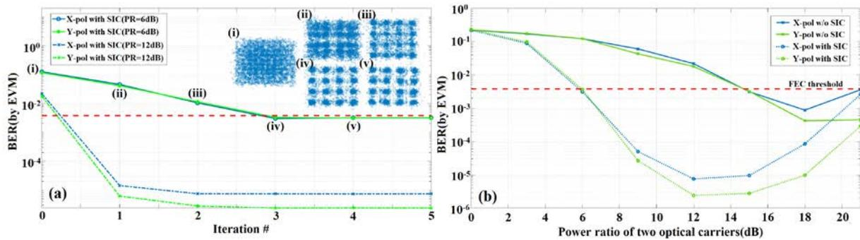
Fig. 3 (a) BER versus SIC iteration number, (b) BER versus the optical carrier power ratios of the PDM signals.
