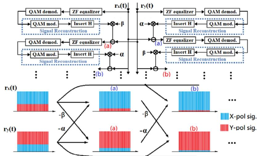
Fig. 1 The conceptual diagram of SIC to eliminate PDM crosstalk.
