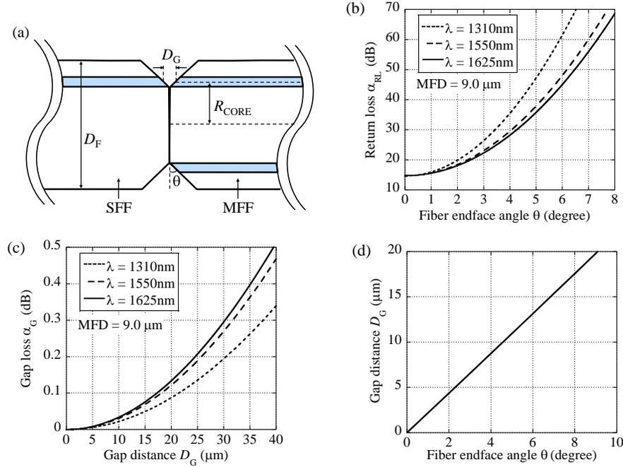
Fig. 2(a) Cross-sectional view of the ferrule aspect inside the sleeve. (b) Relationship between the fiber endface angle and the return loss. (c) Relationship between the gap distance and gap loss. (d) Relationship between the fiber endface angle and gap distance.
