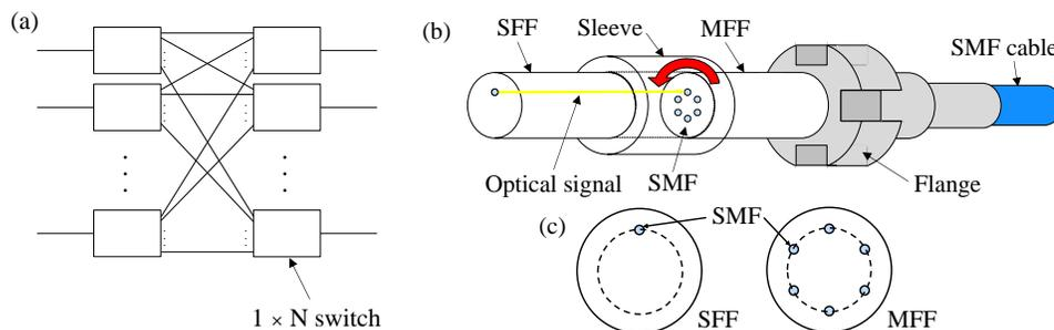
Fig. 1. (a) Optical switch system configuration. (b) Basic arrangement of ferrule rotated optical switching mechanism. (c) Cross-sectional views of SFF and MFF.
