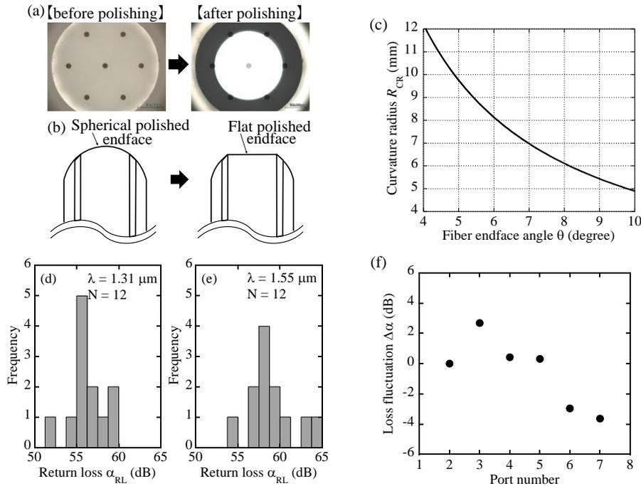
Fig. 3(a) Endface image by microscope observation. (b) Cross-sectional view of ferrule aspect during polishing process. (c) Relationship between fiber endface angle and curvature radius. (d) Return loss characteristics of fabricated MFF at 1.31  $\mu\text{m}$ . (e) Return loss characteristics of fabricated MFF (d) at 1.55  $\mu\text{m}$ . (f) Loss fluctuation by MFF rotated switching.
