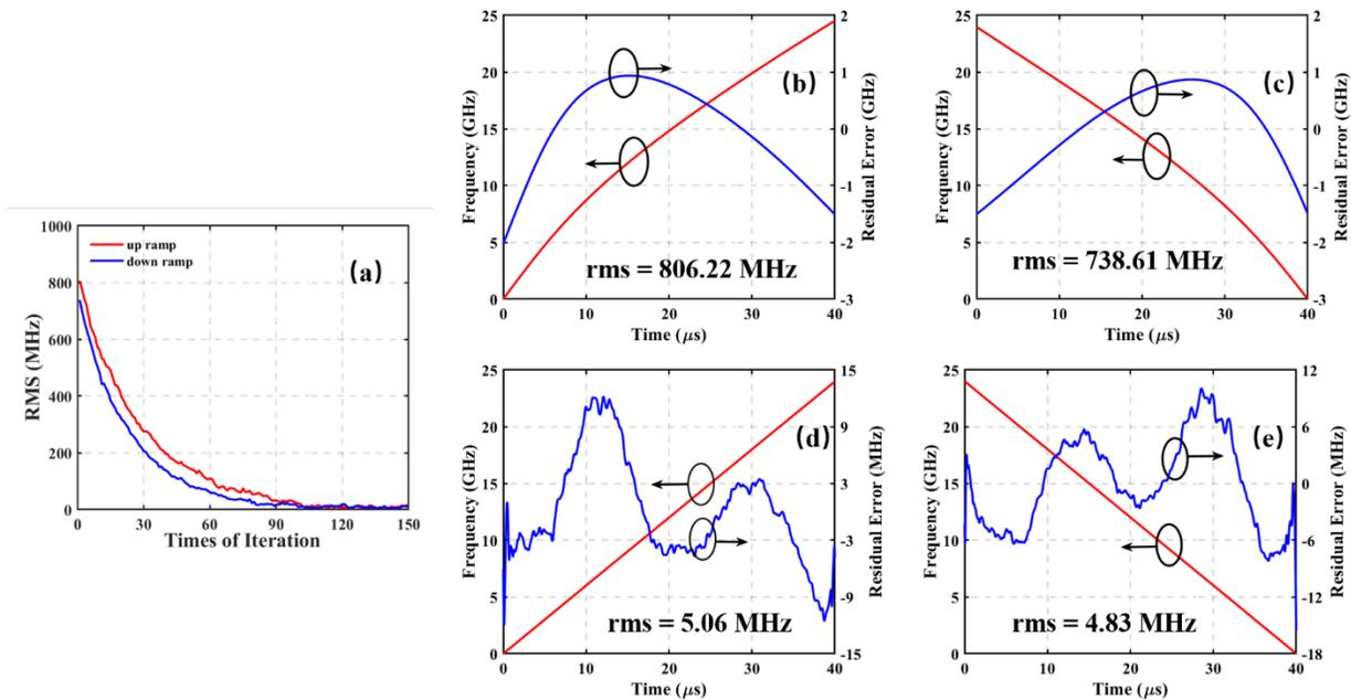
Fig. 4. (a) RMS of the up and down ramps versus the times of iteration; the up- and down-ramp of the laser frequency sweeps and residual error (b)~(c): the initial; (d)~(e): after 136 times of iteration.
