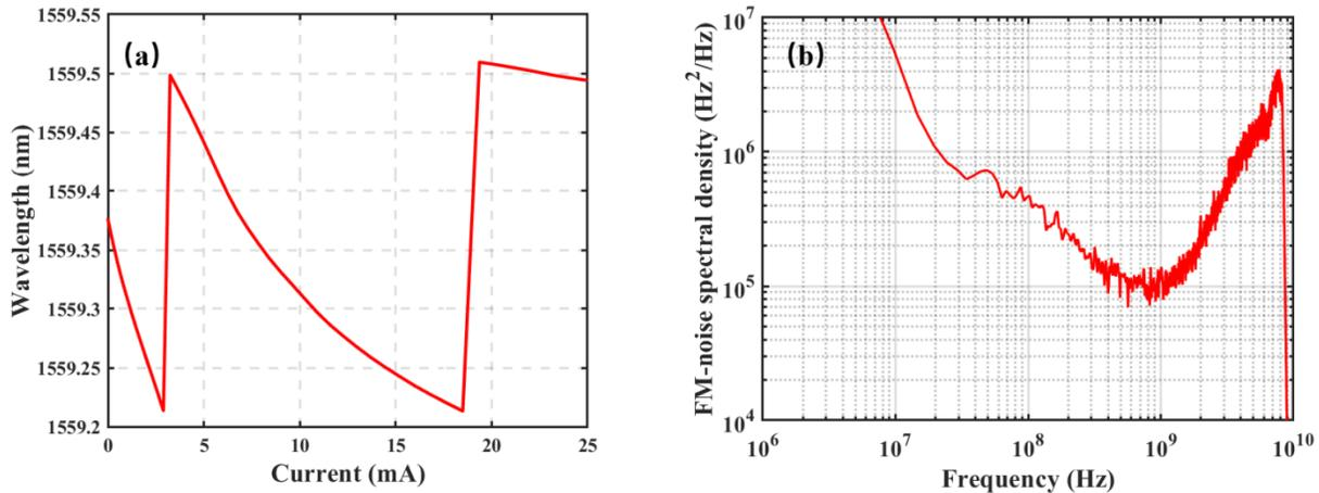
Fig. 3. (a) Wavelength tuning characteristics of the DBR laser when current is injected into the phase region; (b) FM noise spectrum of the DBR laser.
