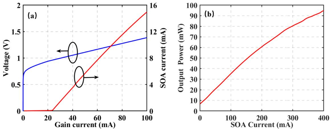
Fig. 2. (a) The LIV curve of the DBR laser; (b) The LI curve when the gain current is 200 mA.
