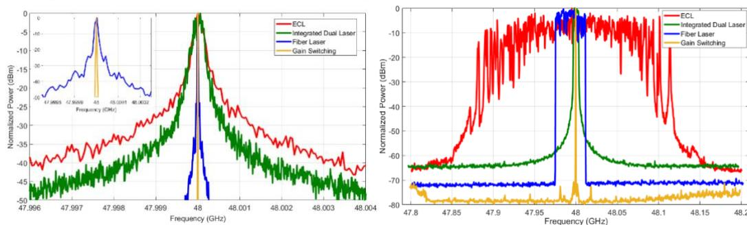
Fig. 2 (a) RF spectra of beat signal using various optical sources for signal generation round 48 GHz (b) RF spectra taken with maximum hold on spectrum analyzer demonstrating large frequency offset fluctuation with discrete sources.
