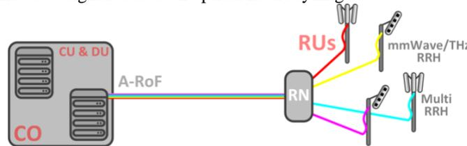
Fig. 1 Centralized radio access network (C-RAN) architecture using ARoF for fronthaul transmission from CO to RU
