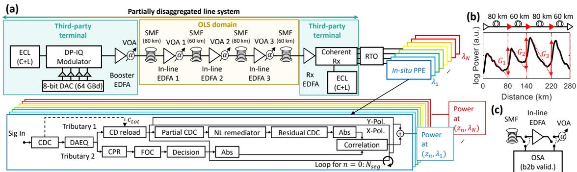
**Figure 1:** (a) Experimental testbed and DSP scheme used in the link tomography. (b) Output of the *in-situ* PPE, where  $G_1$ ,  $G_2$  and  $G_3$  indicate the estimated gain of the 1<sup>st</sup>, 2<sup>nd</sup> and 3<sup>rd</sup> in-line EDFA (at fixed wavelength), respectively. (c) Scheme used for the b2b validation.
