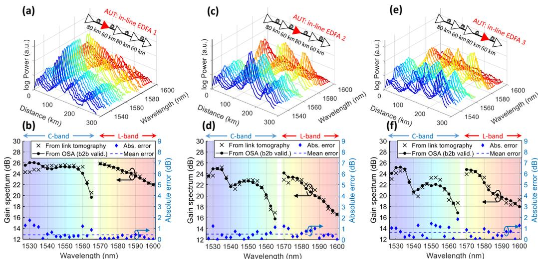
**Figure 2:** Link tomography used to estimate the spectral gain profile in the commissioning mode when the AUT is the in-line EDFA (a) 1, (c) 2 and (e) 3. Estimated gain spectrum for the in-line EDFA (b) 1, (d) 2 and (f) 3. Results obtained for  $\varepsilon = 0.004$ ,  $N_{seg} = 280$ ,  $N = 29$ .
