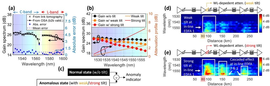
**Figure 3:** (a) Estimated gain spectrum of the AUT 1 in the operation mode. (b) Gain spectra of the AUT 1 without and with emulated gain tilts. (c) Anomaly detection scheme to visualize gain tilt. Anomaly indicator for (d) weak and the (e) strong tilt profiles.
