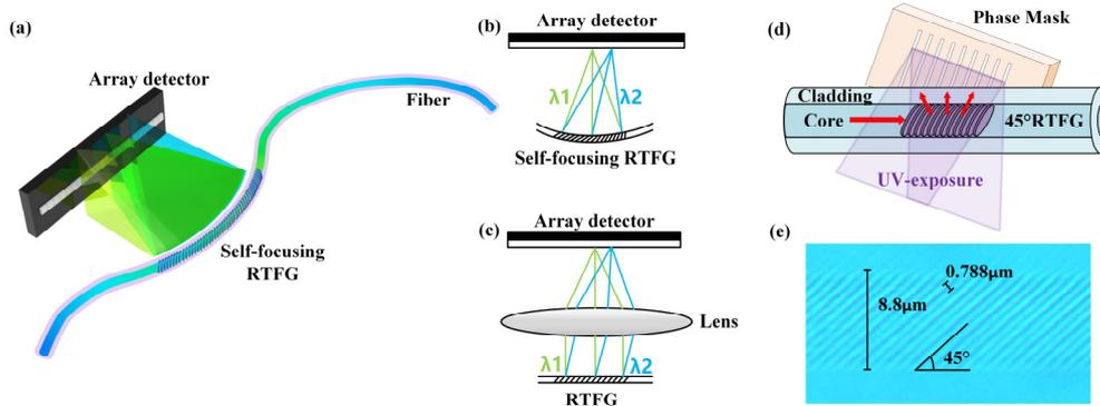
Fig.1 (a) Schematic of the all-fiber micro spectrometer based on self-focusing RTFG, the focusing process of (b) self-focusing RTFG and (c) lens based RTFG, (d) Fabrication of 45° RTFG by UV-exposure and (e) Micrograph of 45° RTFG.
