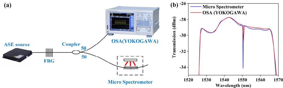
Fig.3 (a) Testing set up for the spectral performance of the all-fiber micro spectrometer, (b) Transmission spectrum.
