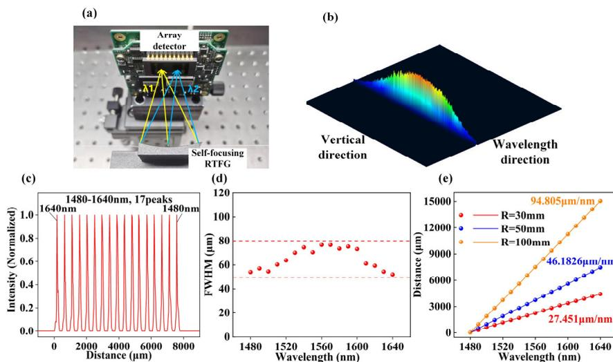
Fig.2 (a) Experimental set up, (b) light distribution on the detector array, (c) measured spectral response, (d) 3-dB bandwidth with different wavelength from 1480 nm–1640 nm and (e) line dispersion curve under different radius of curvature  $R$  (30 mm, 50 mm, 100 mm)
