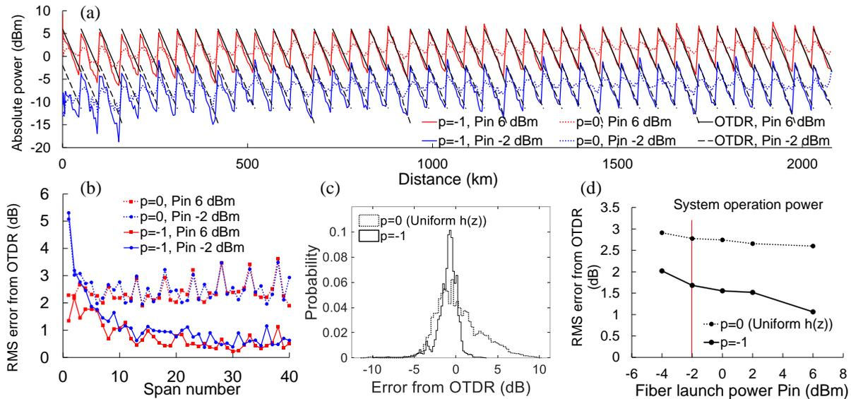
Fig. 3. (a) Estimated power profile ( $p=0, -1$ ) for 2,080 km transmission with fiber launch powers  $P_{in}$  of 6 and -2 dBm. (b) Estimation error of obtained profiles in (a) from theoretical power profiles as a function of span number. (c) Histogram of estimation error from theoretical power profiles at  $P_{in}$  -2 dBm. (d) Estimation error from theoretical power profile as a function of fiber launch power.
