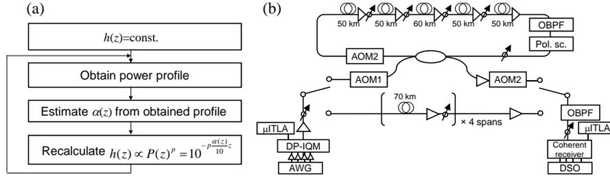
Fig. 1. (a) Proposed step-size optimization scheme for longitudinal power profile monitoring. (b) Experimental setup.
