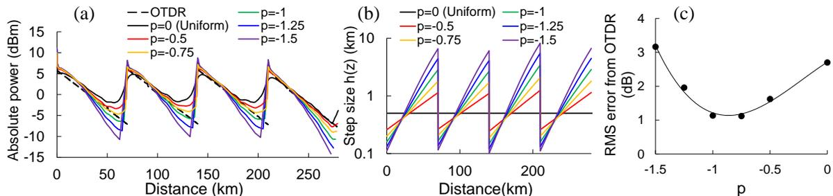
Fig. 2. (a) Estimated power profiles for 280-km transmission with various step size selection rules  $h(z) \propto P(z)^p$ . (b) Step sizes  $h(z) \propto P(z)^p$  for various  $p$ . (c) Estimation error from theoretical power profiles as a function of  $p$ .
